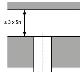
Capacitive sensors must maintain a free zone with the following criteria:
