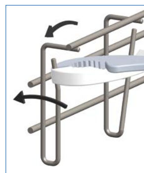
Locking of cables at least cable dimension
