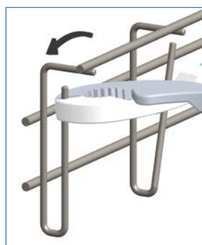
Locking cables at largest cable dimension
