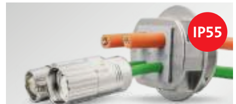
EMC Split cable gland for screw-on assembly with a locknut M32, M63 for cable diameters up to 35 mm
