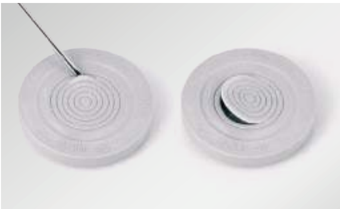
The single membrane rings are peeled off according to the diameter of the routed cable or hose. For this purpose, only a small hole between the rings needs to be pierced. Then the corresponding ring can be removed.
