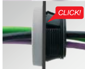
Mounting type 1: Snap into the cut-out For wall thickness 1 – 2.5 mm
