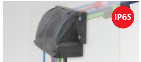
Split flange enclosure for 90° cable transit with integrated seal for cable diameters up to 35 mm
