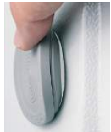
The single membrane rings are peeled off according to the diameter of the routed cable or hose. For this purpose, only a small hole between the rings needs to be pierced. Then the corresponding ring can be removed.
