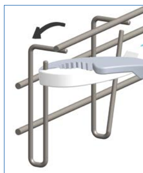
Locking cables at largest cable dimension
