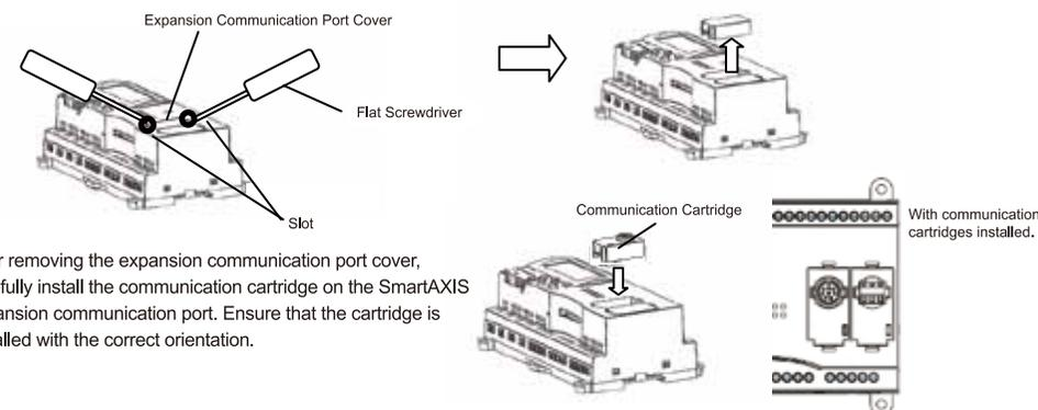
After removing the expansion communication port cover, carefully install the communication cartridge on the SmartAXIS expansion communication port. Ensure that the cartridge is installed with the correct orientation.
