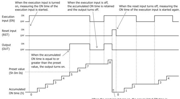
When the reset input turns on, the accumulated ON time is reset to 0 and the output turns off.
