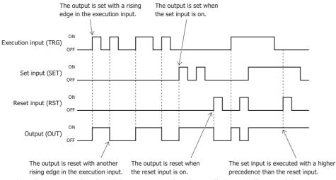
When the set input (SET) and the reset input (RST) are off, the on/off state of the output is inverted at every rising edge in the execution input (EN). The output is also set/reset by the set input/reset input according to the operation mode.
