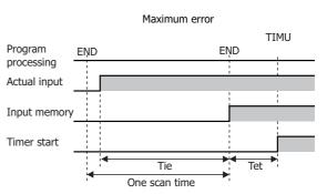
When the actual input turns on immediately after the END processing, Tie  $\approx$  one scan time. In this case, the timer input error is: Tie + Tet  $\approx$  1 scan time + Tet (behind error), and is at its maximum.
