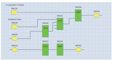
• The initialization input (M0000) turns on with the first scan and the initial settings configured on the P 1 tab are stored in D0000 to D0002.
