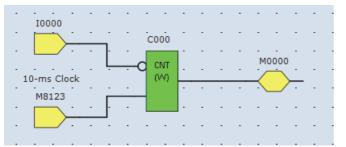
In this case, specify the adding counter (CNT FB) C2 to keep the current value. For details on retaining the current value, see Chapter 5 "Special Functions" – "Keep Designation" in the SmartAXIS Pro/Lite User's Manual.
