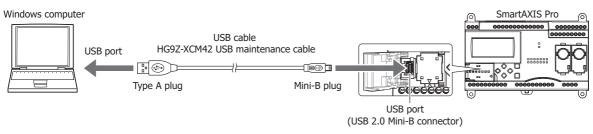
**Note:** To communicate with the SmartAXIS via a USB connection, the dedicated USB driver must be installed in the computer. For the driver installation procedure, see "Appendix" in the "SmartAXIS Pro/Lite User's Manual".
