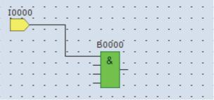
The output connector of the input I0 and the input 1 connector of the AND B0 are connected.
