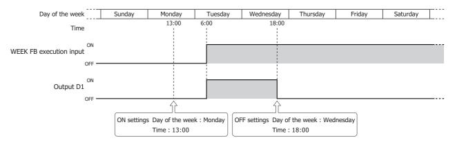
For example, if pulse output is enabled and the ON settings are Sunday 0:00, output D1 turns on and off as follows.
