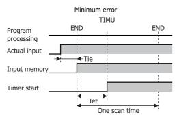
When the actual input turns on immediately before the END processing, Tie  $\approx$  0. In this case, the timer input error is only Tet (behind error), and is at its minimum.
