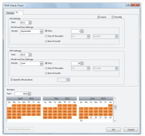
Configure the tabs as shown above and connect the YEAR FB output to Q000.
