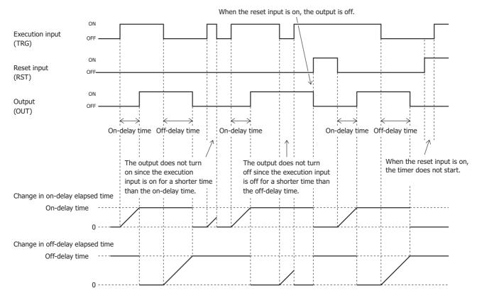
While the reset input (RST) is off and the output (OUT) is off, the current value (on-delay elapsed time) starts being incremented when the execution input turns on.
