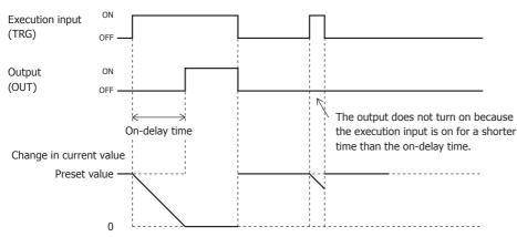
When the execution input (TRG) is off, the current value returns to the preset value (TP) and the output (OUT) is off.
