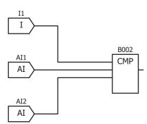
The CMP FB in the above FBD program compares analog input AI1 with AI2 and outputs the result when input I1 is on.
