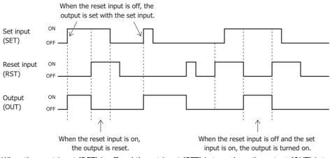
When the reset input (RST) is off and the set input (SET) is turned on, the output (OUT) is turned on. The output state is maintained even after the set input is turned off. Once the reset input (RST) is turned on, the output is turned off. When the reset input is on, the output is not turned on even if the set input is turned on. When the set input and the reset input are both on and the reset input is turned off, the output is turned on.
