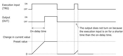
When the execution input (TRG) is off, the current value is 0 and the output (OUT) is off.
