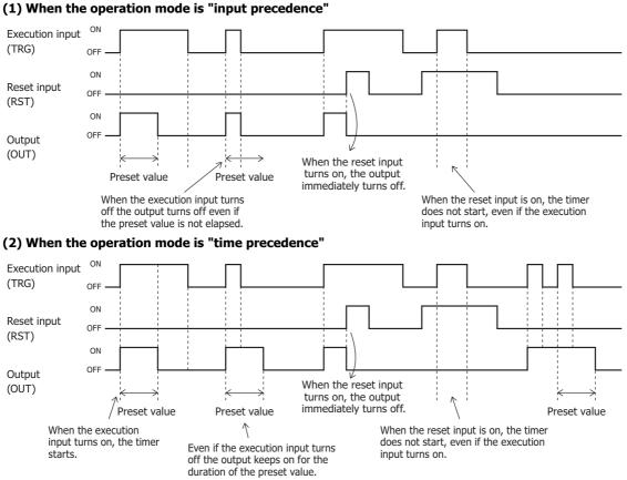
When the execution input (TRG) turns on while the reset input (RST) is off, the current value returns to 0, the output turns on, and the current value starts being incremented. When the current value reaches the preset value (TP), the output (OUT) turns off. The FB operation depends on the operation mode, when the execution input turns off while the current value is being incremented.
