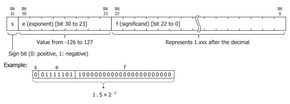
The table below shows the correspondence between values in the three fields of s, e, and f, and the value expressed as a single precision floating point value. When a value other than a normal number or 0 is input to a FB that uses floating point, a user program execution error occurs and special internal relay M8004 (user program execution error) turns on.
