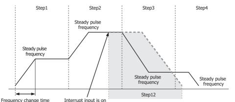
An external input (I0 to I35) or internal relay (M0 to M1277) can be specified as the interrupt input.
