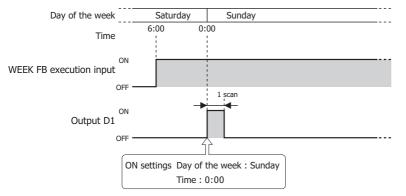
During the period from Sunday 0:00:00 to 0:00:59, when the WEEK FB execution input changes from OFF to ON, output D1 turns ON for only one scan. (In this diagram the WEEK FB execution input is turned on at 0:00:30 on Sunday)
