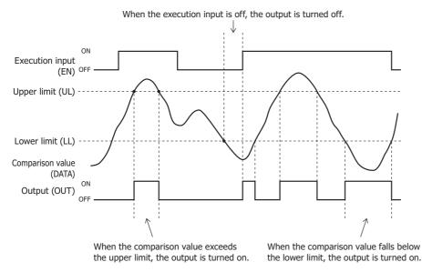
When the execution input (EN) is on, the output (OUT) is turned on/off as described below.
