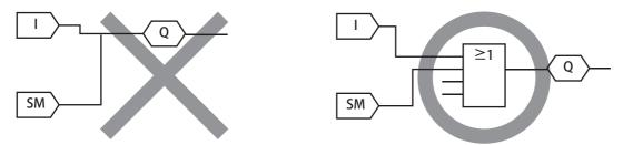
The FB output connector can be connected to more than one input connectors of the other FBs. There is no limit to the number of input connectors that an output connector can be connected to.
