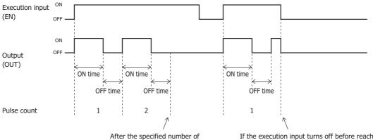
pulses are output, pulse output stops.
