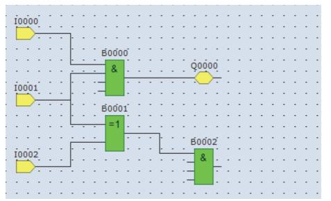
**Note:** A single FB output connector can be connected to multiple FB input connectors. Multiple FB output connectors cannot be connected to a single FB input connector.
