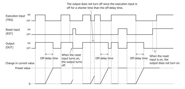
When the execution input (TRG) turns on while the reset input (RST) is off, the current value returns to 0 and the output (OUT) turns on.
