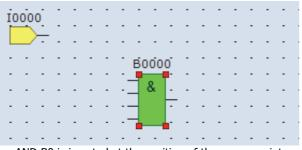
AND B0 is inserted at the position of the mouse pointer.
