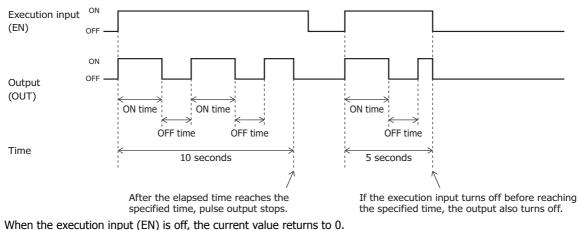
When the execution input (EN) is on, the current value returns to 0. When the execution input (EN) turns on, the current value (ON time elapsed time) starts being incremented. According to the operation mode, the output is on for the duration of ON time (TP1) and off for the duration of OFF time (TP2).
