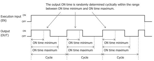
If "continuance" is selected as the operation mode, the on/off operation of pulse output (i.e. pulse output) is repeated at the specified cycle (TP3) while the execution input is on. The output turns on for a random time within the range of time between ON time minimum and ON time maximum, and then the output turns off for the remaining time of the cycle. When the execution input turns off, the output turns off.
