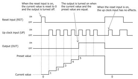
When the reset input is off, the counter is in the countable state. While the counter is in the countable state, it increments the current value at every rising edge in the up clock input.
