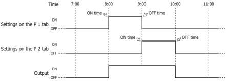
• If ON time is 9:00 and OFF time is 10:00 on the P 1 tab and ON time is 8:00 and OFF time is 9:00 on the P 2 tab, the 9:00 setting is duplicated on the 2 tabs and ON time for the P 1 tab is disabled. In this situation, the output is on from 8:00 to 9:00.
