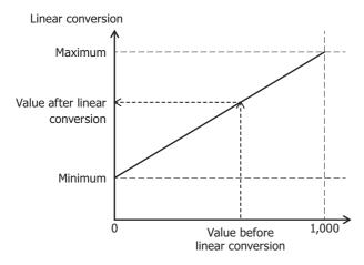
Example: When the minimum is -5,000 and the maximum is 10,000, an analog input value of 600 is linearly converted into 4,000.
