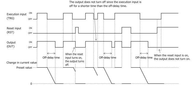
When the execution input (TRG) turns on while the reset input (RST) is off, the current value returns to preset value and the output (OUT) turns on.
