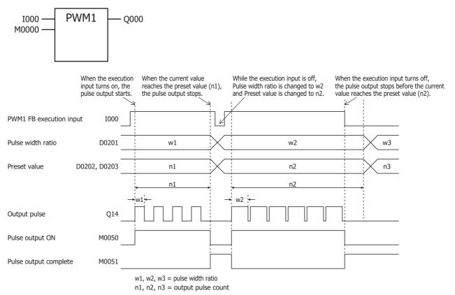
• When the PWM1 FB execution input (I0) turns from off to on, M50 turns on and pulses are output with the width ratio configured by D201.
