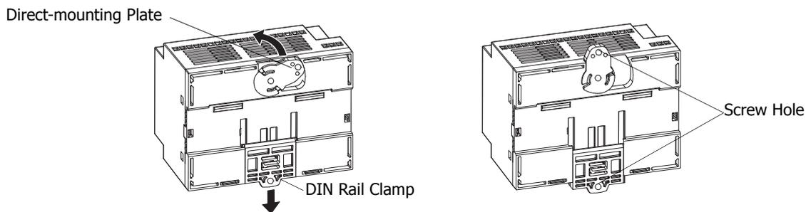
**Mounting Hole Layout for Direct Mounting on Panel Surface**
