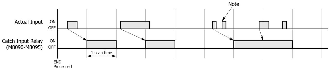
**Catching Falling Edge of Input Pulse**
