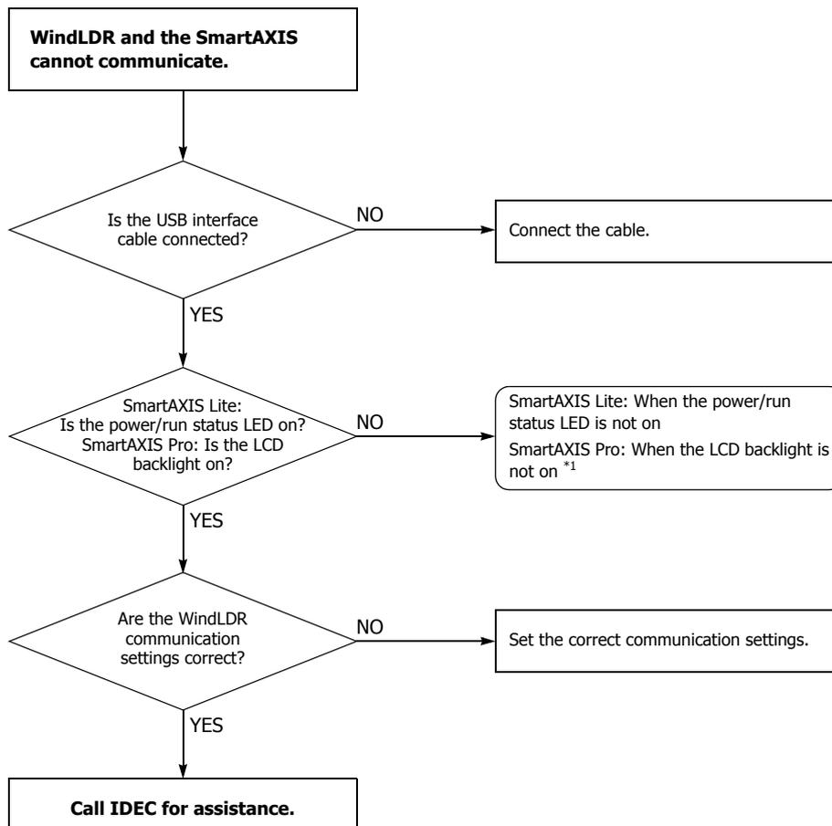
\*1 See "SmartAXIS Pro - The Backlight is not On" on page 14-9 or "SmartAXIS Lite - The Power/Run Status LED (PWR/RUN) is not On" on page 14-10.
