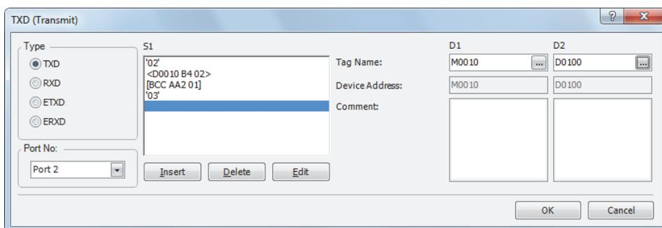
Programming of the TXD2 instruction is complete and the transmit data is specified as follows:
