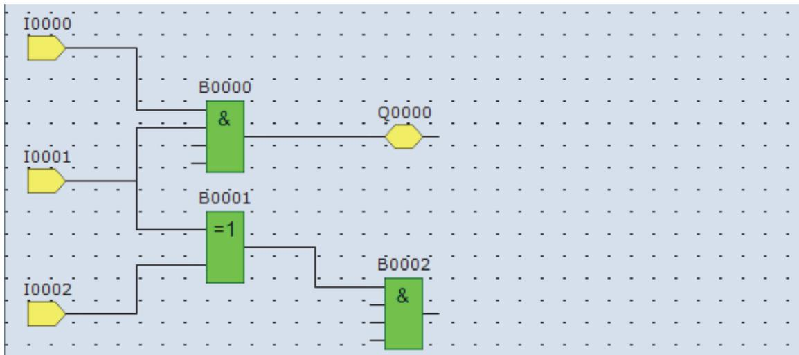
The output connector of the FB can be connected to multiple FB input connectors. Multiple output connectors of FBs cannot be connected to a single input connector of an FB.
