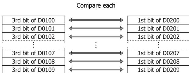
**Note:** Even if the data type is set to D (double word), L (long), or F (float), the comparison is performed from the starting device in bit units.
