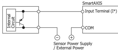
**Output Terminal Wiring**
