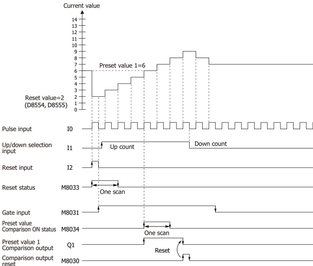
1. When reset input (I2) turns on, the reset value (D8054, D8055) is stored in the current value (D8050, D8051). In this situation, reset status (M8033) turns on for only one scan.
