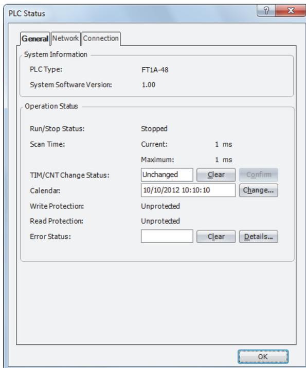
You can check the SmartAXIS system software version with **System Software Version**.
