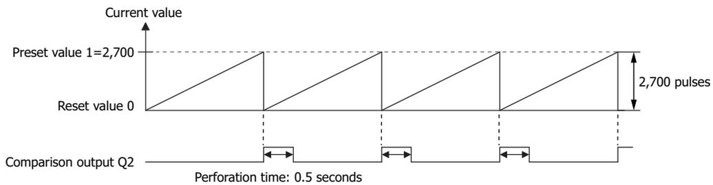
**Note:** In this example, Z-phase reset input is not used.
