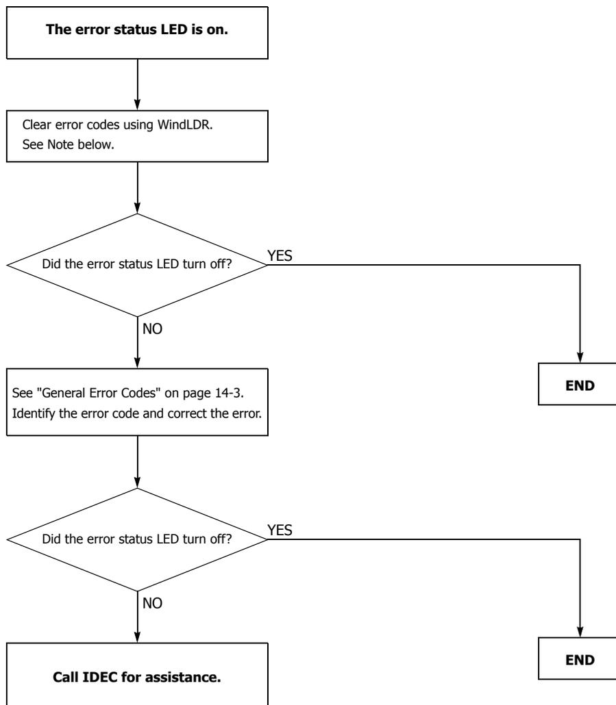
**Note:** Temporary errors can be cleared to restore normal operation by clearing error codes from WindLDR. See "Clearing Error Codes from WindLDR" on page 14-2.
