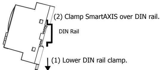
3. Align the SmartAXIS with the DIN rail and raise the DIN rail clamp.
