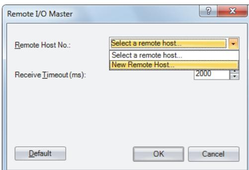
4. Configure the IP address and port number of the remote I/O slave to connect.
