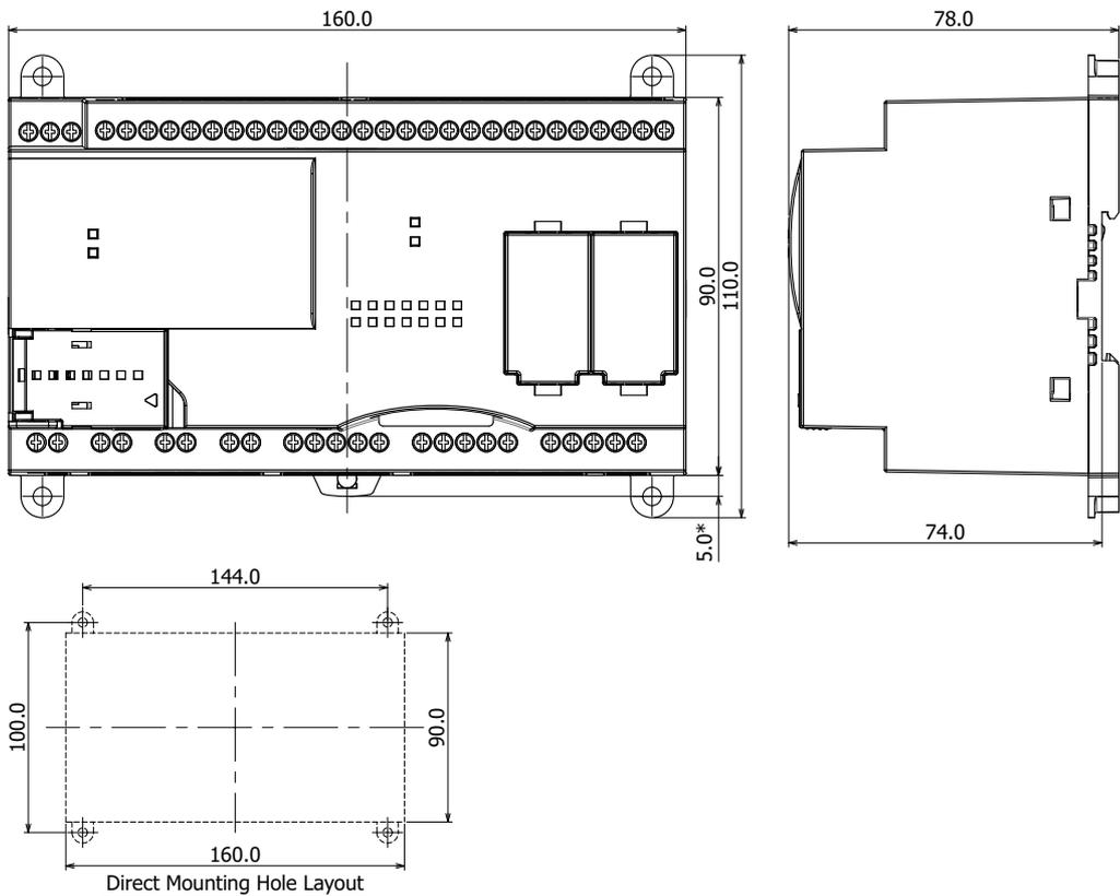
\*9.3mm when the clamp is pulled out.
