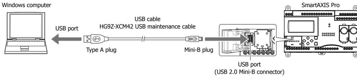
**Note:** In order for WindLDR to communicate with the SmartAXIS via USB, a dedicated USB driver must be installed on the computer. See "USB Driver Installation Procedure" on page A-5.
