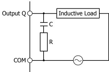
This protection circuit can be used when the load impedance is smaller than the RC impedance in an AC load power circuit.
