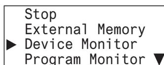
3. Select device type: M (internal relay) with the ◀ (left) and ▶ (right) buttons and press and hold the **OK** (OK) button. **0** flashes to indicate the focus is on M0000.
