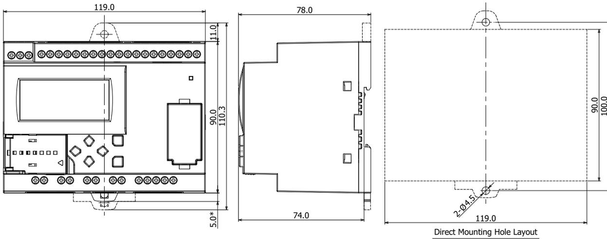
\*9.3mm when the clamp is pulled out.
