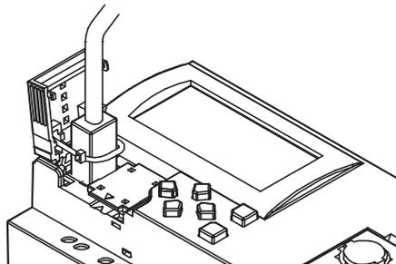
4. Tighten the loop until it is the suitable size and trim the excess cable tie using wire cutters.
