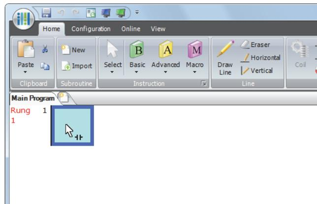
**Note:** Another method to insert a NO (or NC) contact is to move the mouse pointer where you want to insert the contact, and type A (or B). The Normally Open dialog box appears.
