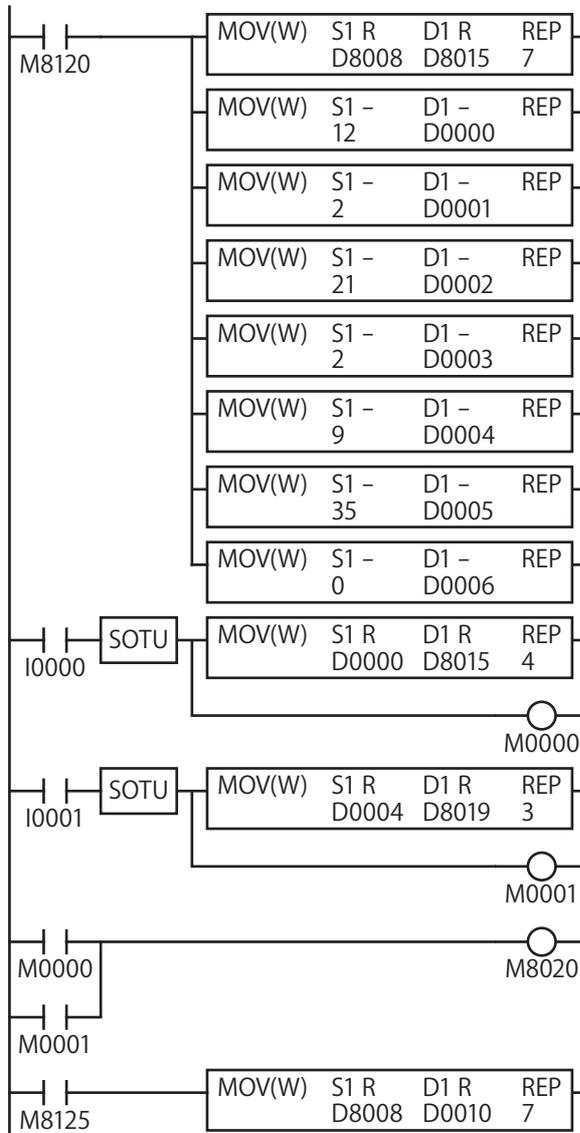
M8120 is the initial pulse that turns on for only one scan at the start of operation.
