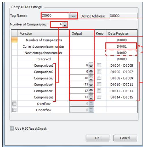
The data register that stores the preset value (target value). Specify the starting address.
