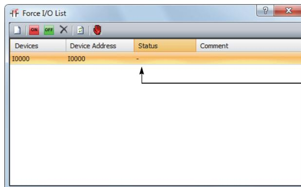
Input I0 is released from the forced I/O designation. Even when forced I/O is enabled, actual input status is read to the SmartAXIS.
