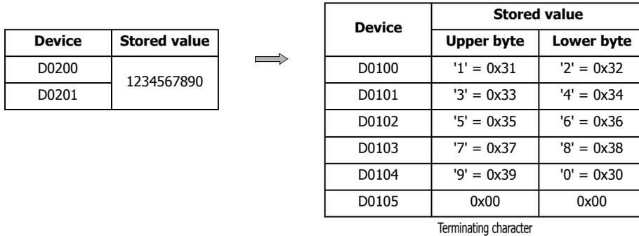
**Converting -1234567890 (when the data type is L (long))**
