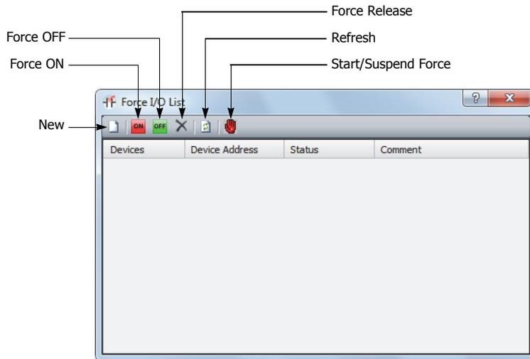
3. Click the New button and type an input or output number under Device in the list.
