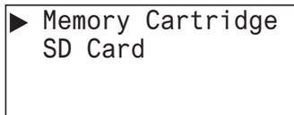
4. Select **PLC -> Cartridge** with the (up) and (down) buttons and press the (OK) button.
