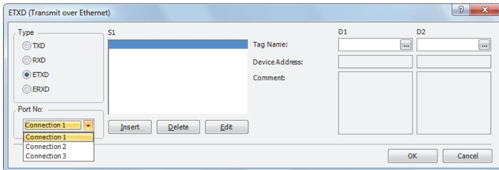
Select ETXD (Transmit over Ethernet) to transmit data or ERXD (Receive over Ethernet) to receive data as the instruction type. Select the client connection from 1 through 3 and designate S1, D1, and D2. Click **OK** button to close the dialog box.
