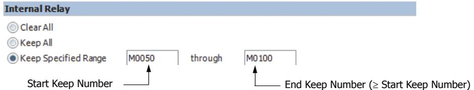
When a range of M50 through M100 is designated as shown in the example above, M50 through M100 are keep types, M0 through M47 and M101 through M1277 are clear types.
