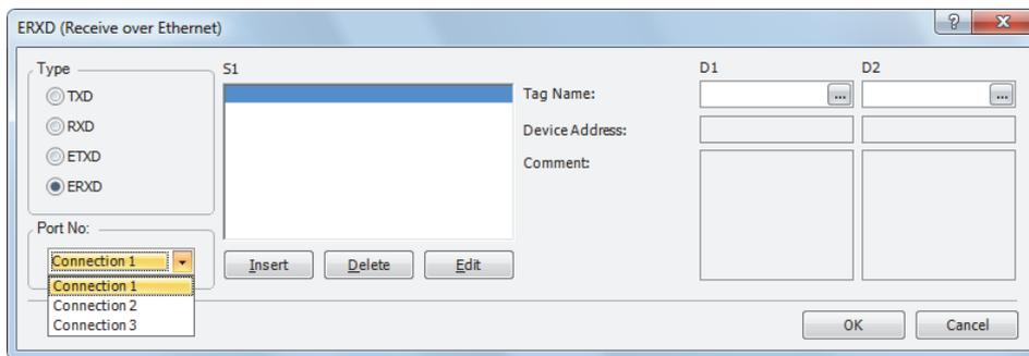
Select **ETXD** (Transmit over Ethernet) to transmit data and **ERXD** (Receive over Ethernet) to receive data as the instruction type. Select the server connection from 1 through 8 and designate S1, D1, and D2. Click **OK** button to close the dialog box.
