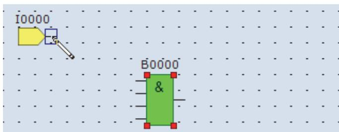
3. Click the left mouse button and drag the line to the AND B0 input 1 connector.
