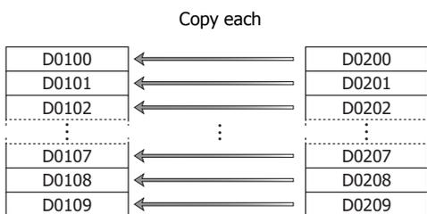
**Note:** Even if the data type is set to D (double word), L (long), or F (float), the data is copied from the starting device in word units.
