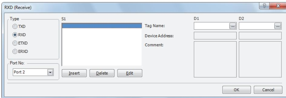
2. Check that **RXD** is selected in the Type box and select **Port 2** in the Port box. Then, click **Insert**. The Data Type Selection dialog box appears. You will program source device S1 using this dialog box.
