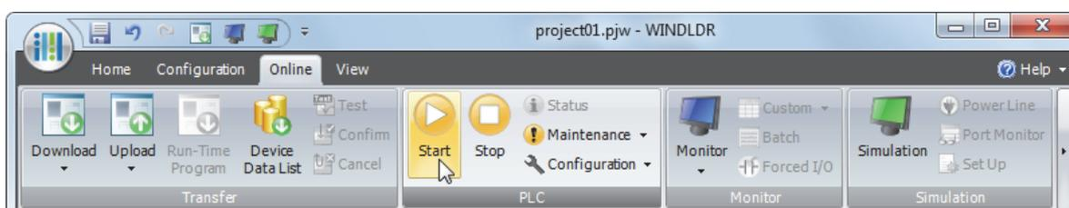
4. Click the **Start** button to start operation, then the start control special internal relay M8000 is turned on.
