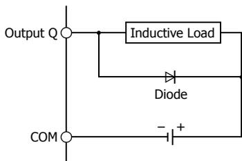
This protection circuit can be used for DC load power circuits.
