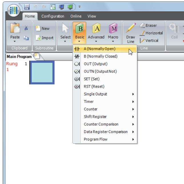
2. Move the mouse pointer to the first column of the first line where you want to insert a NO contact, and click the left mouse button.
