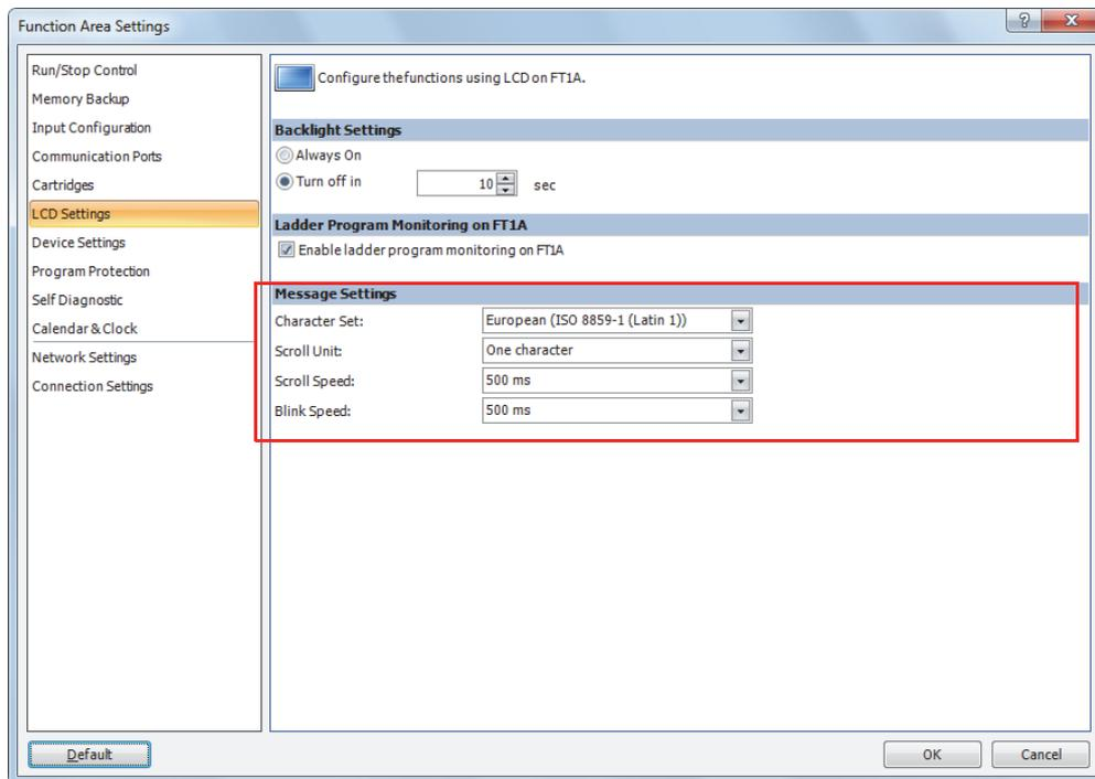
2. Configure the character set, scroll unit, scroll speed, and blinking speed in the message settings.
