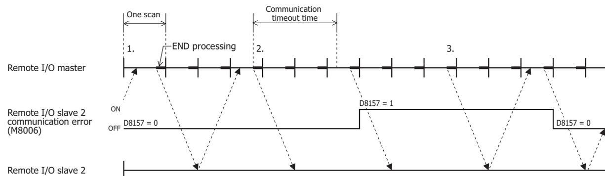
1. While communicating with the remote I/O slave, the remote slave communication error (M8005 to M8007) is off and the remote slave communication error status (D8148, D8157, D8166) is "0" (normal).
