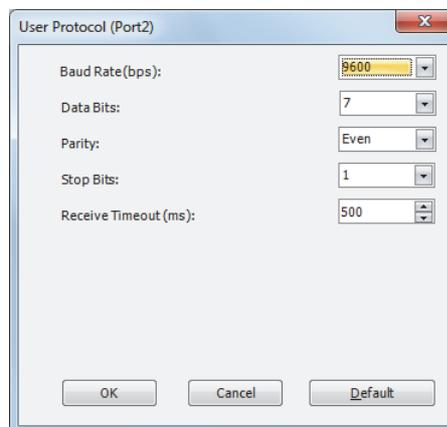
When **2550ms** is selected in the Receive Timeout box, the receive timeout function is disabled.
