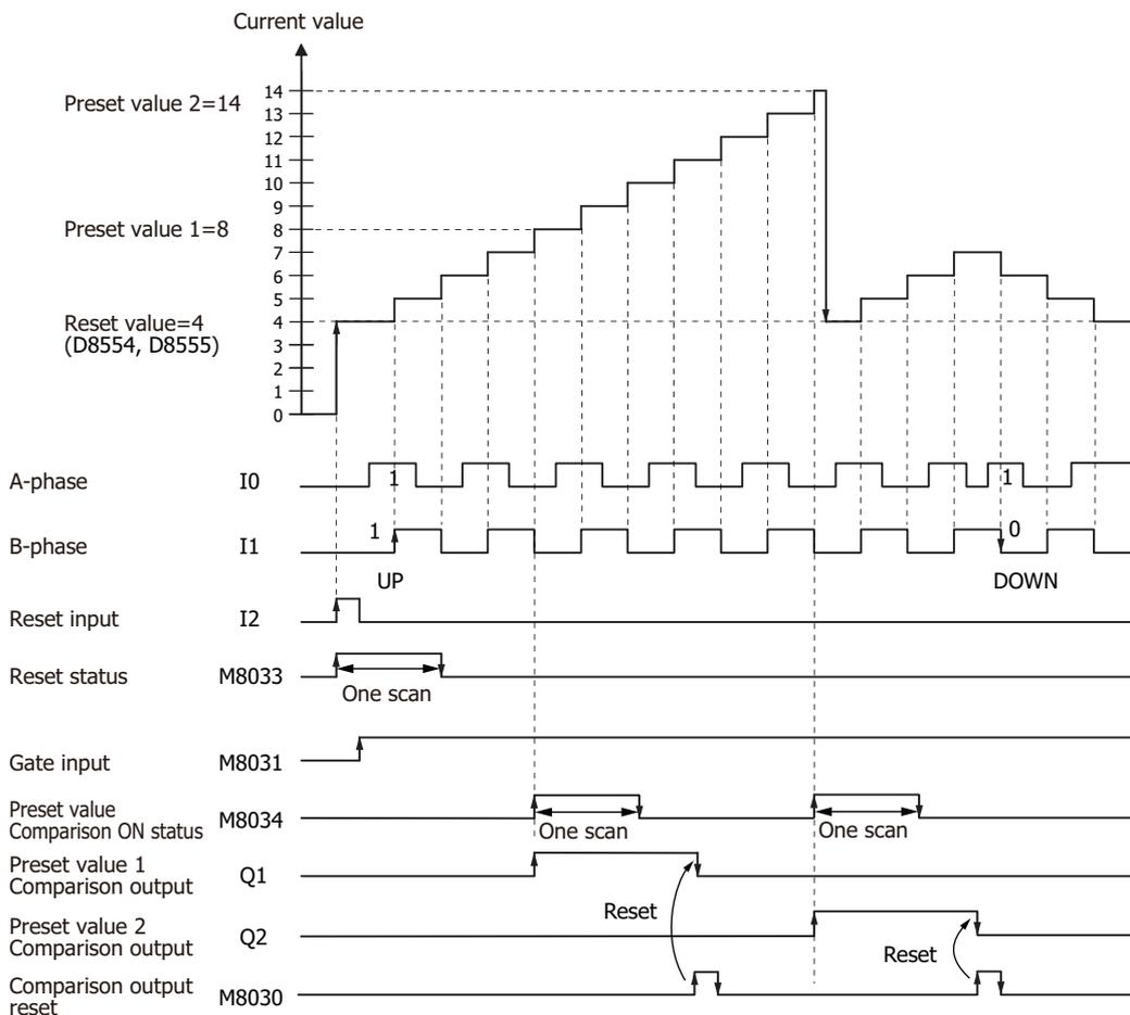
1. When reset input (I2) turns on, the reset value (D8054, D8055) is stored in the current value (D8050, D8051). In this situation, reset status (M8033) turns on for only one scan.
