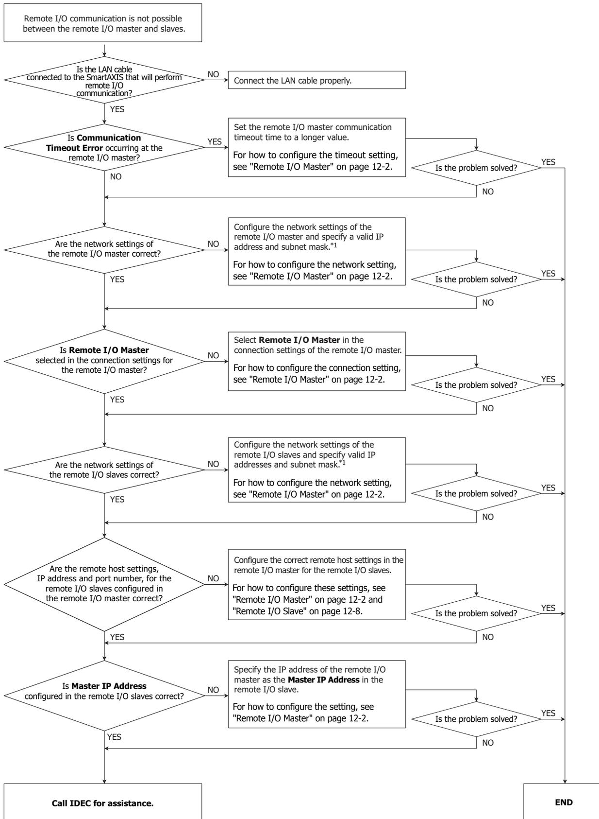
\*1 Use valid network settings, IP address, subnet mask, and port number, for the remote I/O communication. For the valid network settings for the SmartAXIS, contact the network administrator.
