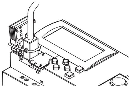
3. The cable tie can also be inserted through the holes on the USB port cover.
