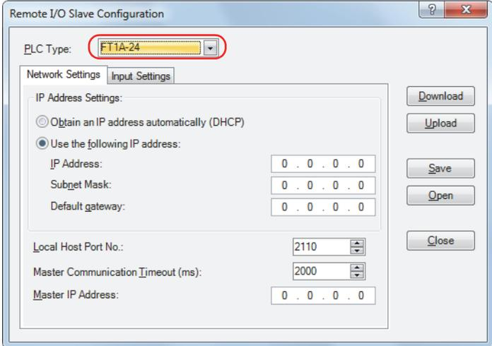
3. Click the **Network Settings** tab and configure the IP address, subnet mask, default gateway, local host port number, and master communication timeout for the remote I/O slave.
