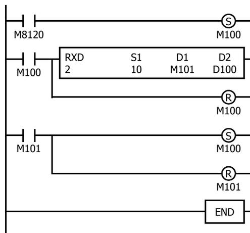
M8120 is the initialize pulse special internal relay used to set M100.
