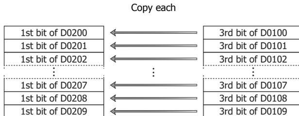
**Note:** Even if the data type is set to D (double word), L (long), or F (float), the bits are copied from the starting device in bit units.
