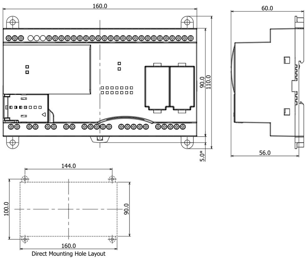
\*9.3mm when the clamp is pulled out.
