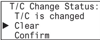
The changes made to the timer and counter preset values are deleted. The preset values of the user program in the ROM remain as they are before those values are modified. The device values return to the values before they are modified.
