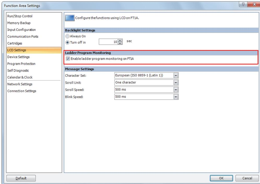
2. Select the **Enable ladder program monitoring on FT1A** check box.
