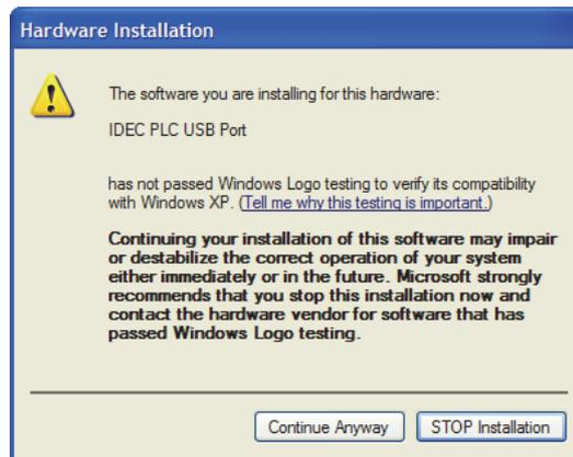
If the installation is aborted without showing the dialog box above, **Block** is selected in the Driver Signing Options in **Driver Signing** in the **System Properties** dialog box. If the installation is aborted, this option should be changed to **Warn**. After changing the option to **Warn**, reconnect the SmartAXIS and retry the installation procedure from the step 1.
