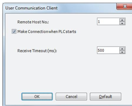
Configure the remote host number and receive timeout. If you want the SmartAXIS to establish the connection when it starts to run, select "Make Connection when PLC starts." Click **OK** button to close the dialog box.
