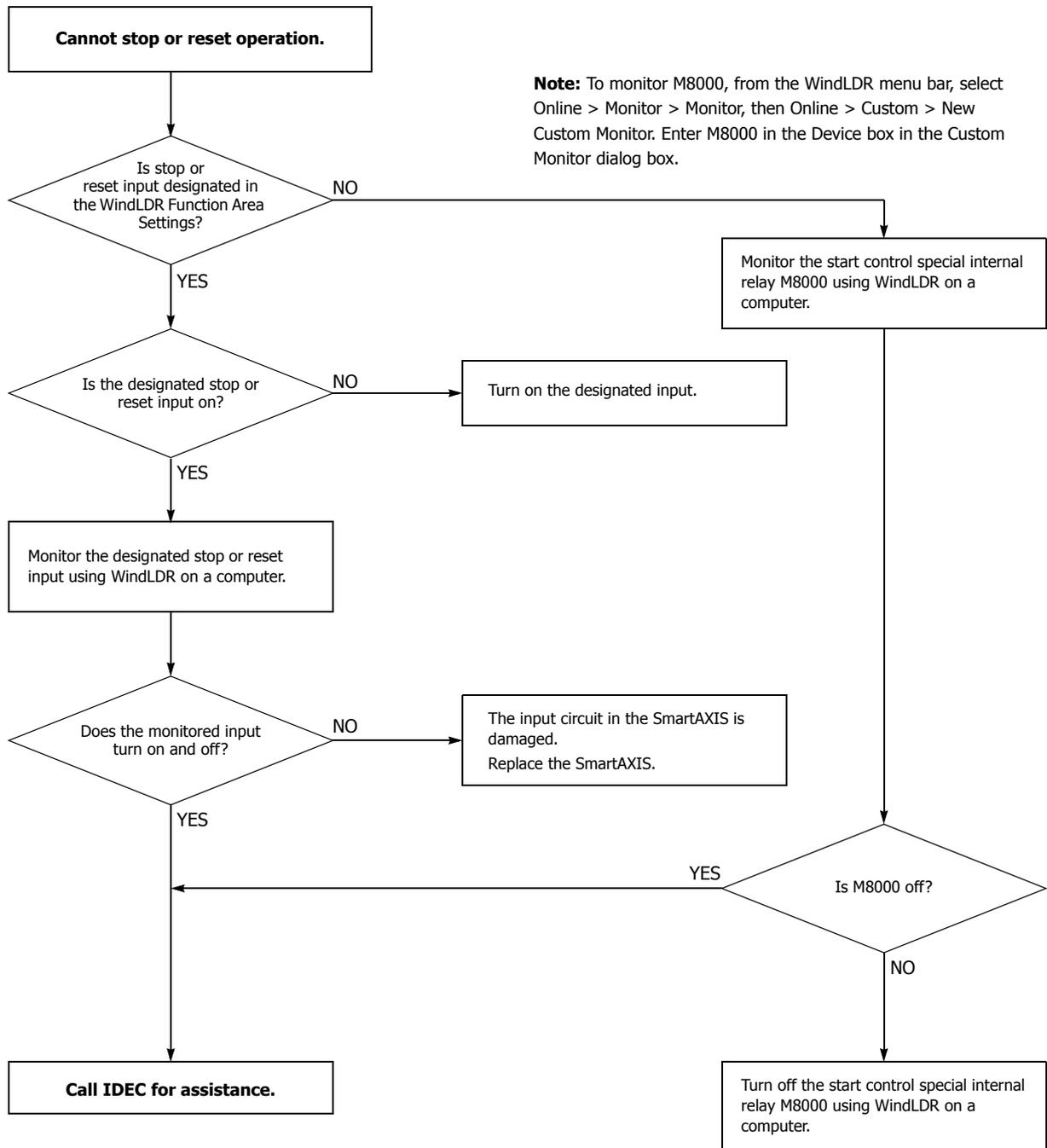
**Note:** To monitor M8000, from the WindLDR menu bar, select Online > Monitor > Monitor, then Online > Custom > New Custom Monitor. Enter M8000 in the Device box in the Custom Monitor dialog box.
