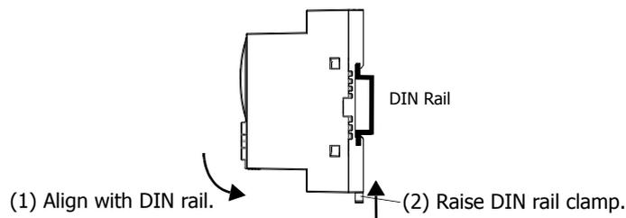
4. Secure both ends of the SmartAXIS using the DIN rail brackets.
