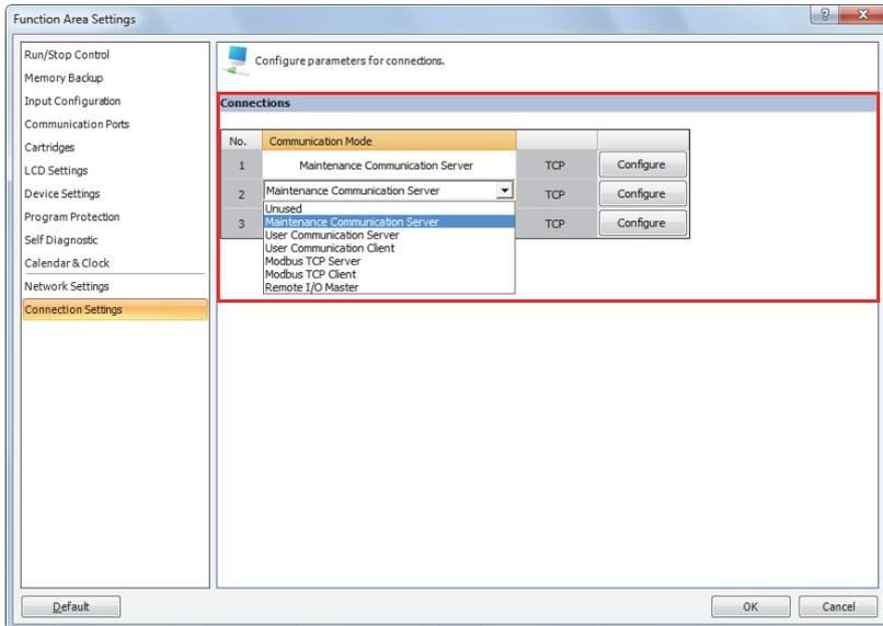
Configure the communication mode allocated to a maximum of three connections that can be used as client or server. Each connection can be set to a different port number. Set connections that are not used to **Unused**.
