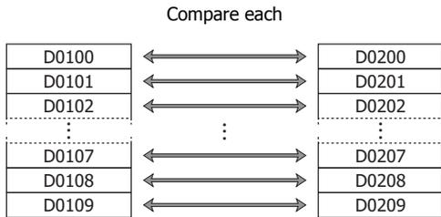
**Note:** Even if the data type is set to D (double word), L (long), or F (float), the comparison is performed from the starting device in word units.
