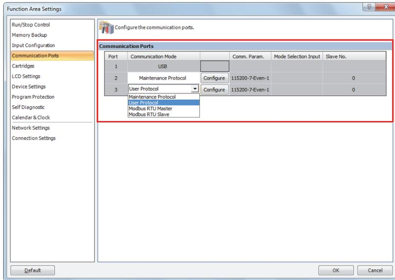
3. Change the settings on the configuration dialog according to the communication format for the destination device.
