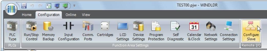
2. Click **PLC Type** and select the PLC type of the connected SmartAXIS to configure.
