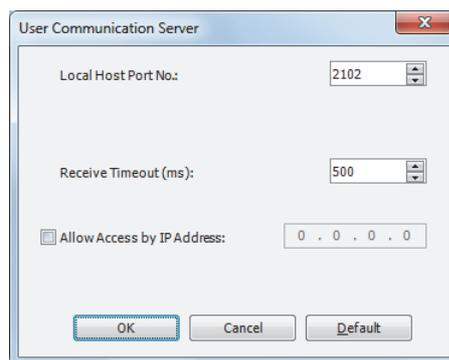
Configure the local host port number and receive timeout. If you want to restrict the access using IP address, configure the allowed IP address.
