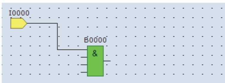
The output connector of the input I0 and the input 1 connector of the AND B0 are connected.
