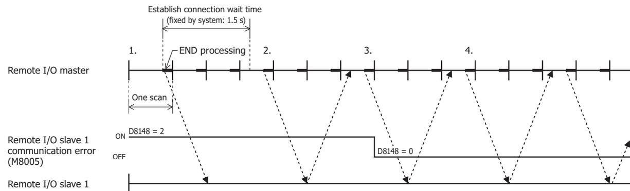
The remote I/O master issues a communication request to the remote I/O slave in the END processing.
