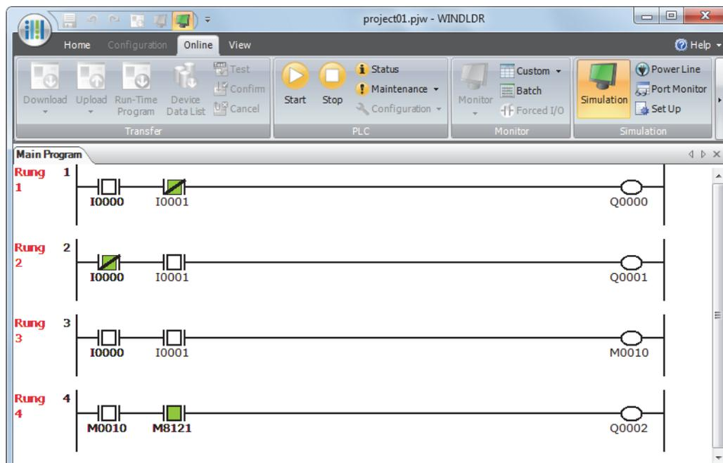
To change an input status, place the mouse pointer on the input and right-click the mouse. In the pop-up menu, select Set or Reset to set or reset the input.
