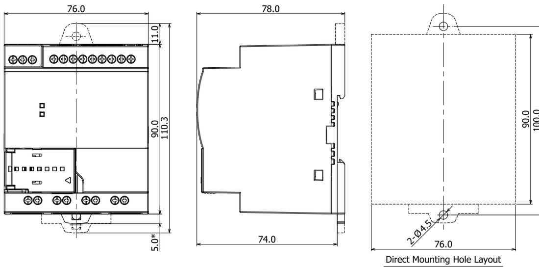
\*9.3mm when the clamp is pulled out.
