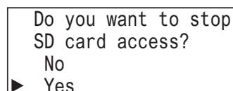
6. While the access to the SD memory card is being stopped, the screen below is displayed. When stopping the access is finished, the screen in step 4 is displayed.
