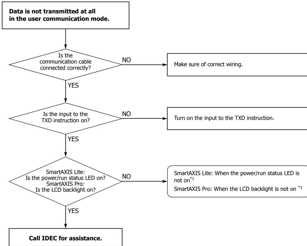
\*1 "SmartAXIS Pro - The Backlight is not On" on page 14-9 or "SmartAXIS Lite - The Power/Run Status LED (PWR/RUN) is not On" on page 14-10.
