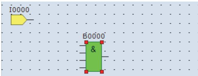
AND B0 is inserted at the position of the mouse pointer.
