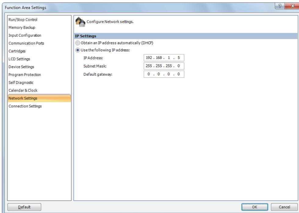
2. Select **Obtain an IP address automatically (DHCP)** or **Use the following IP address**.
