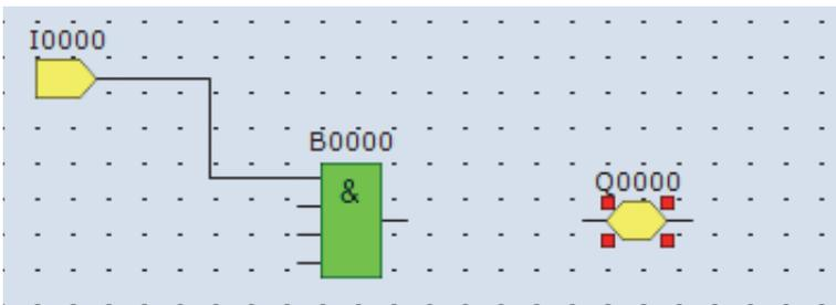
Output Q0 is inserted at the position of the mouse pointer.
