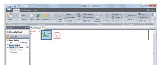
3 Set the device in the **Property** window. Enter "I1" for **Device** and press ENTER. A NC contact of input I1 is programmed in the first column of the first ladder line.
