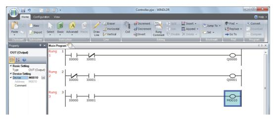
2 A new ladder line is inserted.
