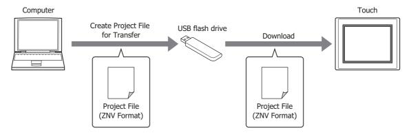
• Upload the project data used for operation on the Touch and save it to an external memory.
