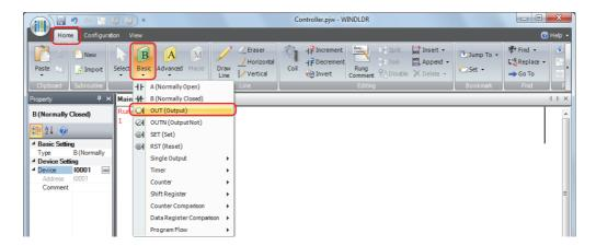
2 Move the mouse pointer to the third column of the first ladder line where you want to insert an output coil, and then click the left mouse button.
