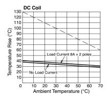
The above temperature rise curves show characteristics when 100% the rated coil voltage is applied.
