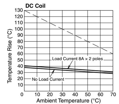
The above temperature rise curves show characteristics when 100% the rated coil voltage is applied.
