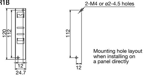
When installed on switching power supply
