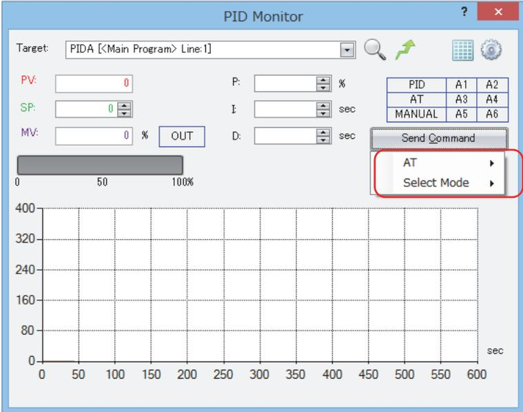
When a PIDD instruction is selected, you can send the following commands to the FC6A Series MICROSmart: Change PID control mode (manual/auto/cascade), enable/disable self tuning, enable/disable PV tracking, proportional gain dependent/independent, enable/disable derivative control, and enable/disable derivative decay. Click this button to display a popup menu and click the corresponding item to send the command.
