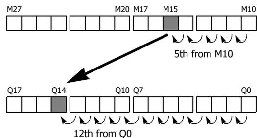
If the current value of counter C5 assigned by destination device D2 is 12, the destination is determined by adding the offset value to output Q0 assigned by destination device D1.
