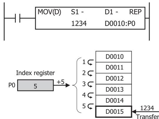
Values stored in the index registers is 32-bit and its data type is L (long). Index registers can directly specified as source and destination devices in MOV(L), ADD(L), SUB(L), and MUL(L) instructions and values in index registers can be moved or manipulated.
