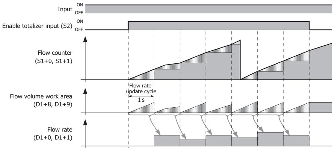
**Note:** For details on the flow calculation function such as the operation immediately after the input is turned on and the operation when the enable totalizer input is once again turned on, see "Flow Rate Function" on page 27-20.
