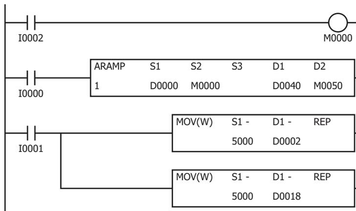
When I2 turns on, the initialization input (M0000) is turned on and the ARAMP instruction control register values are initialized
