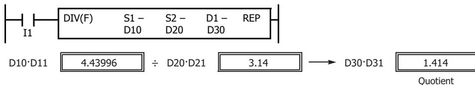
**Note:** Since the destination uses two word devices in the division operation of float data, data register such as D7999 cannot be used as destination device D1.
