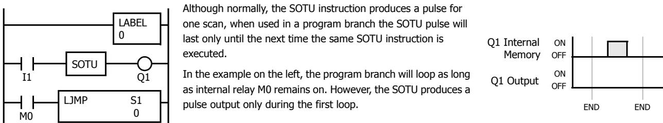
Since the END instruction is not executed as long as M0 remains on, output Q1 is not turned on even if input I1 is on.
