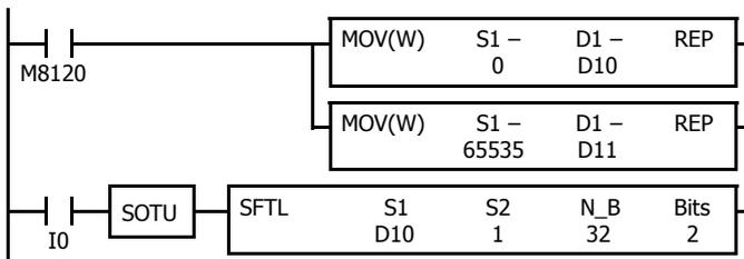
M8120 is the initialize pulse special internal relay.
