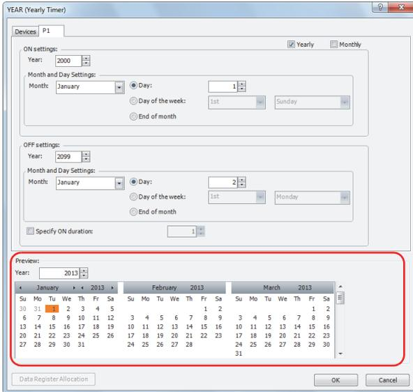
The preview shows the ON/OFF state for the output based on the settings configured on the parameter tabs in a calendar. The dates that are set to ON are highlighted in orange. Three months are shown at one time.
