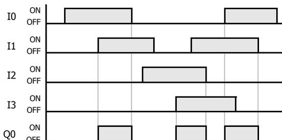
When both inputs I0 and I1 are on or when both inputs I2 and I3 are on, output Q0 is on.
