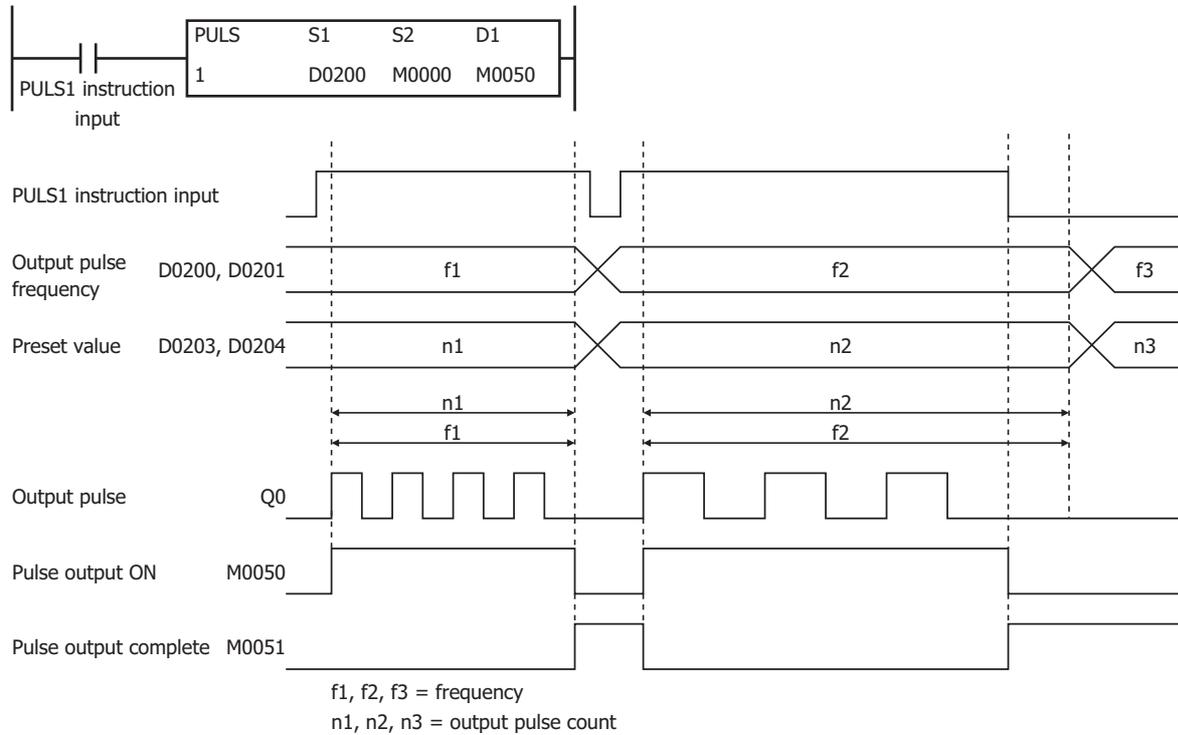
When the PULS1 instruction input changes from off to on, M0050 turns on and pulses with the frequency configured by D0200 and D0201 are output. When the number of pulses configured by D0202 and D0203 are output, pulse output stops. If the value of D0200 and D0201 changes during pulse output, pulses are output with the frequency based on that value.
