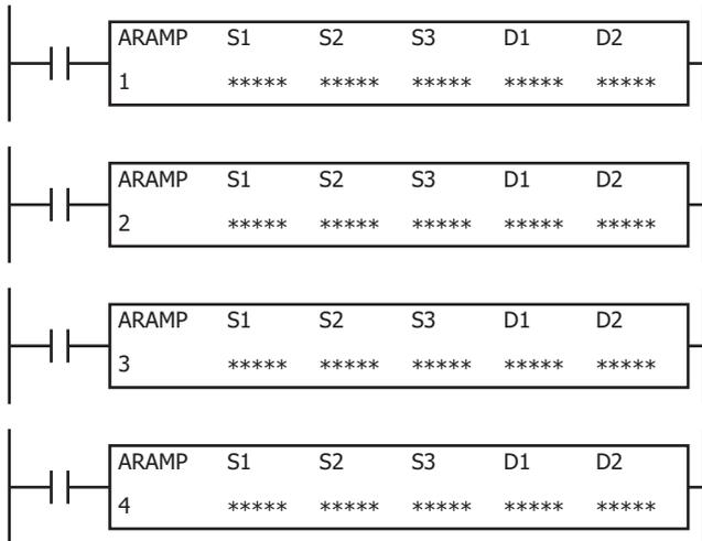
The ARAMP instructions output pulses with the frequency change function according to the information in the frequency table.
