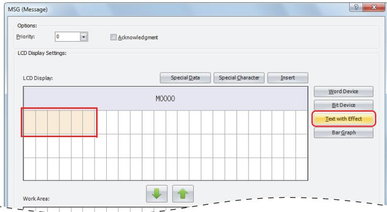
**Note:** The text can also be entered directly on the LCD display area. In the sample above, move the cursor to the start of the second line and enter "Now:" with the keyboard. When you directly enter the text, proceed to "Configuring the word device" on page 12-13, step 8. The **Insert Text with Effect** dialog box is displayed.
