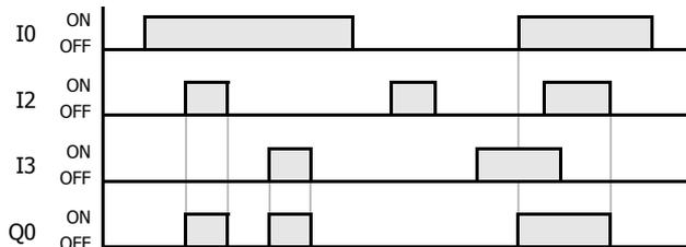
When input I0 is on and either input I2 or I3 is on, output Q0 is on.
