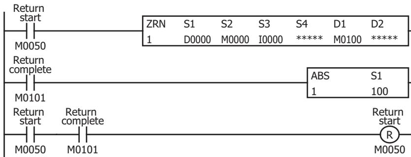
After the power is turned on, the ZRN1 instruction is started and a zero return is performed.
