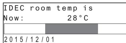
When M0000 is off, the outdoor temperature stored in D0002 is displayed as the numeric value (°C) and bar graph.
