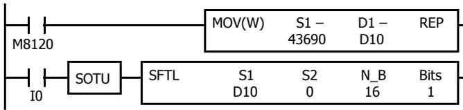
M8120 is the initialize pulse special internal relay.
