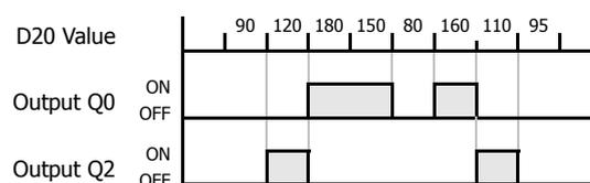
Output Q2 is on while data register D20 value is between 149 and 100.
