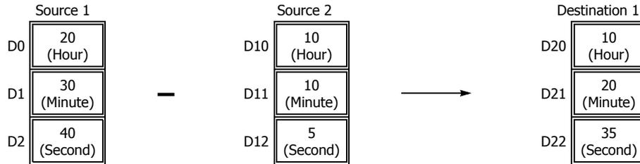
When the result is less than 00:00:00, 24 is added to the result, turning on special internal relay M8003 (borrow).
