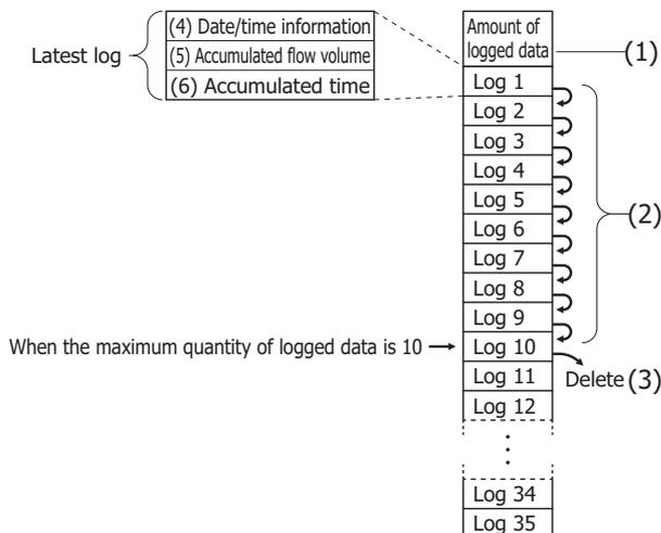
The maximum amount of logged data to use is specified on the **Settings** tab in the **FLWP (Pulse Flow Totalizer)** dialog box.
