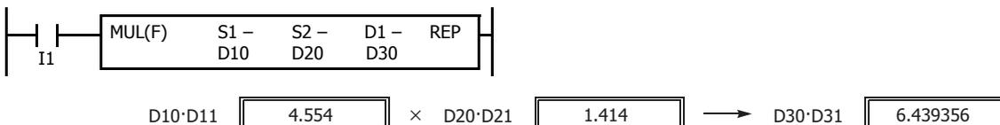
**Note:** Since the destination uses two word devices in the multiplication operation, data register such as D7999 cannot be used as destination device D1. When using a bit device such as internal relay for destination, 32 internal relays are required; so internal relay such as M7961 cannot be used as destination device D1.
