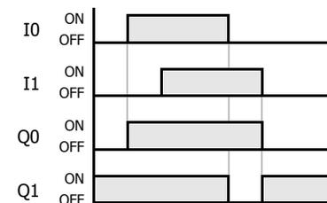
When either input I0 or I1 is on, output Q0 is on. When both inputs I0 and I1 are off, output Q0 is off.
