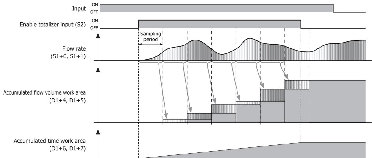
**Note:** For details on the totalizer function such as the operation immediately after the input is turned on and the operation when the enable totalizer input (S2) is once again turned on, see "Totalizer Function" on page 27-11.
