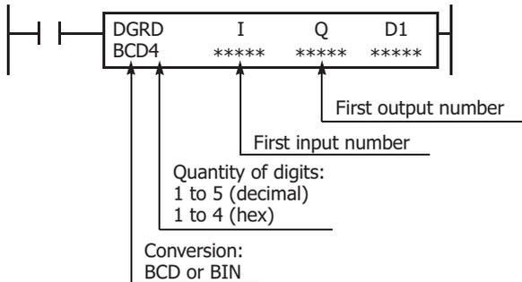
When input is on, the setting values for the connected digital switch are stored in the device specified by D1.
