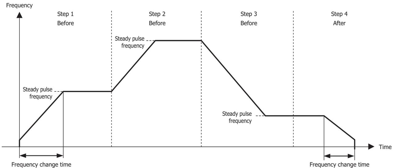
When the initialization input specified by S2 is turned on, the initial values configured in the WindLDR **ARAMP (Ramp Pulse Output with Table)** are stored in the control registers.
