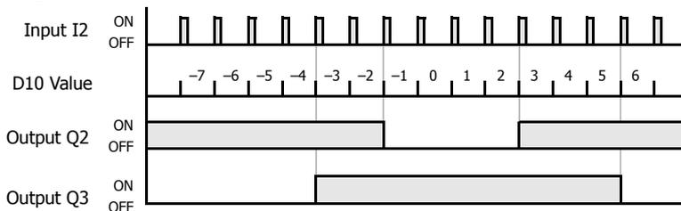
Output Q2 is on when data register D10 is less than or equal to -2 and greater than or equal to 3.
