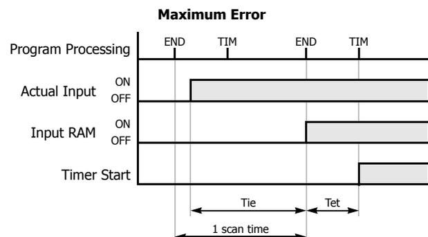
When the input turns on immediately after END processing, Tie is almost equal to one scan time. Then the timer input error is Tie + Tet = one scan time + Tet (behind error) and is at its maximum.
