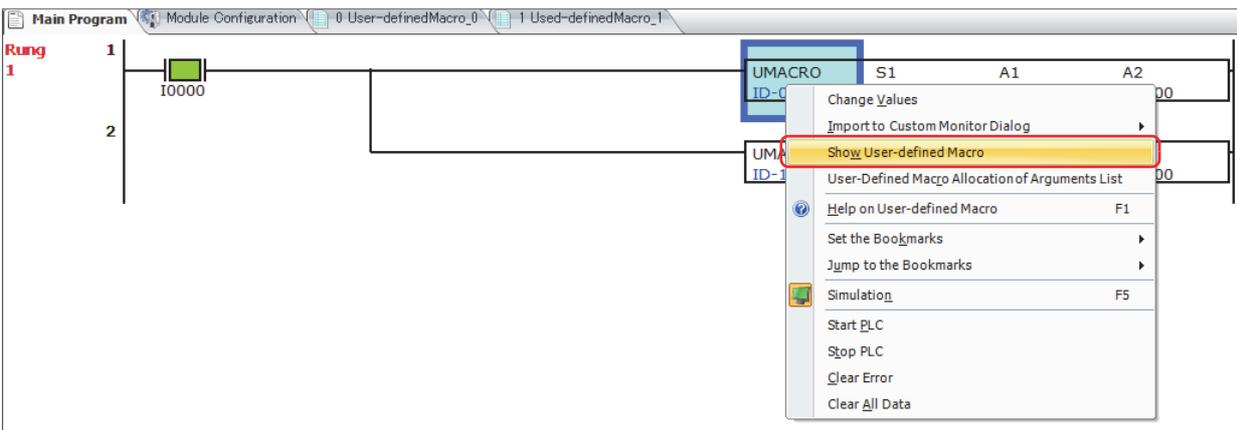
3. The user-defined macro opens that has the number set for the UMACRO instruction. The set argument devices (A1 to A100) are simulated and monitored according to the status of the device address or tag name set for the UMACRO instruction that called the user-defined macro.
