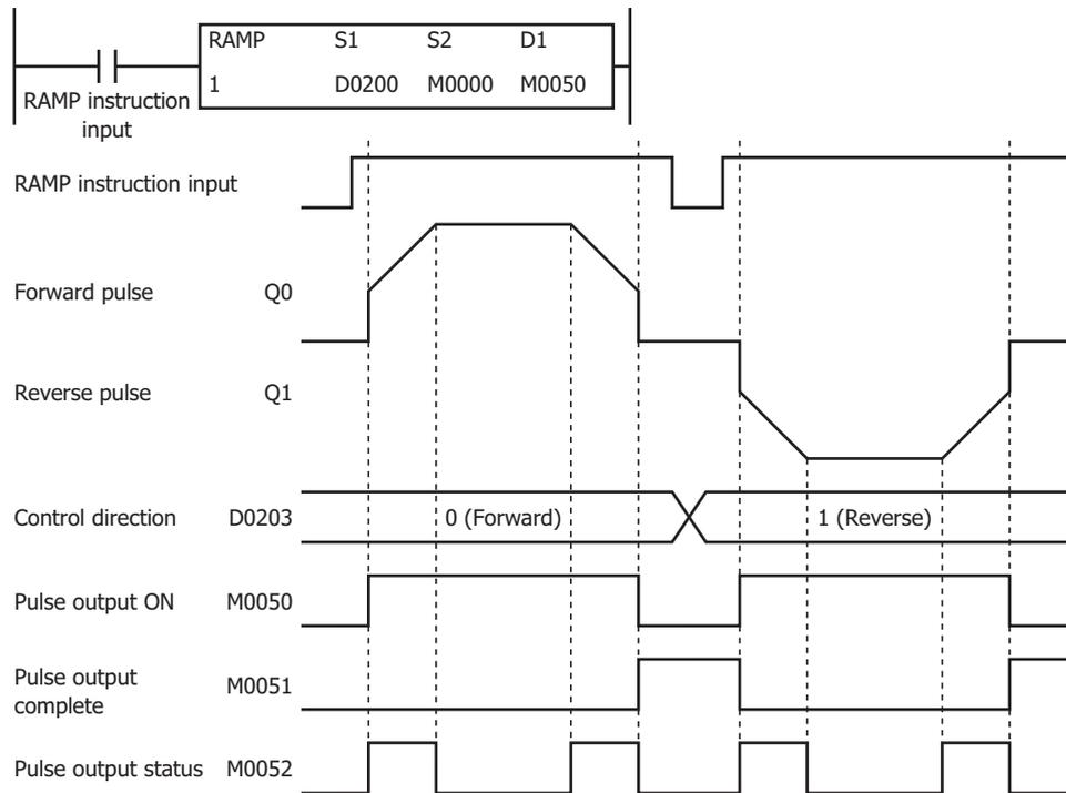
When the RAMP instruction input changes from off to on, pulses are output from Q0 or Q1 according to the settings configured by the control registers.
