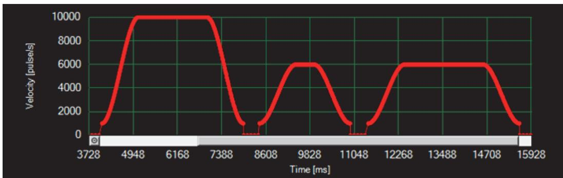
**Example of Simultaneous Dual Axis Control Using the RAMPL Instruction**
