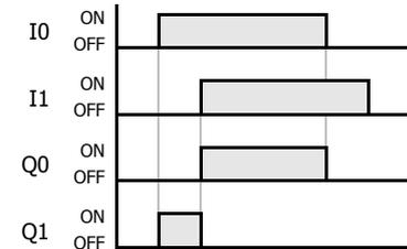
When both inputs I0 and I1 are on, output Q0 is on. When either input I0 or I1 is off, output Q0 is off.
