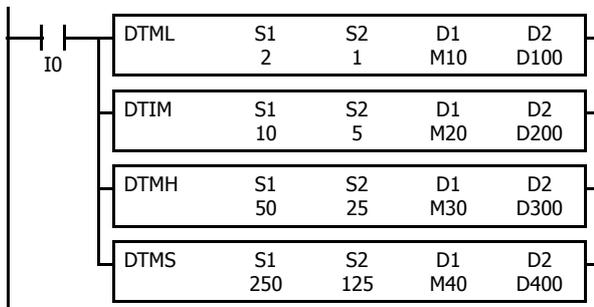
While input I0 is on, four dual timer instructions turn on and off the destination devices according to the on and off durations assigned by source devices S1 and S2.
