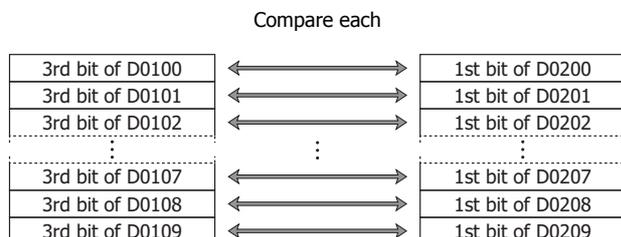
**Note:** Even if the data type is set to D (double word), L (long), or F (float), the comparison is performed from the first device in bit units.
