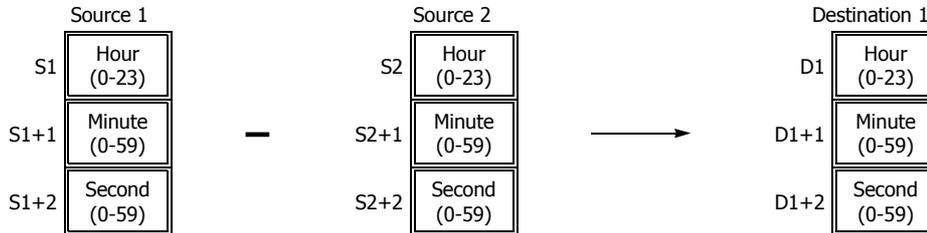
Hour data can be 0 through 23. Minute and second data can be 0 through 59.
