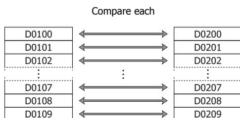
**Note:** Even if the data type is set to D (double word), L (long), or F (float), the comparison is performed from the first device in word units.
