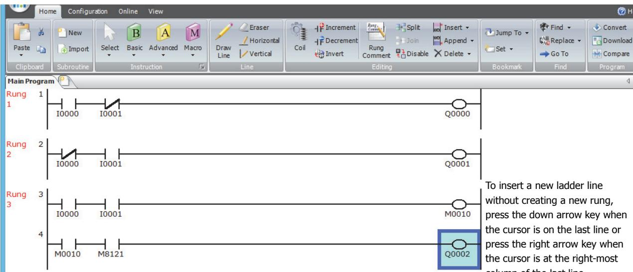
To insert a new ladder line without creating a new rung, press the down arrow key when the cursor is on the last line or press the right arrow key when the cursor is at the right-most column of the last line.
