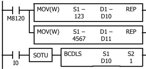
M8120 is the initialize pulse special internal relay.
