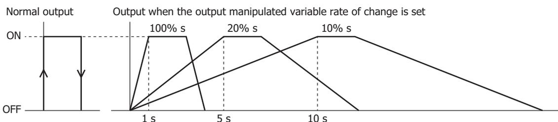
This function is suitable for the control of high-temperature heaters (elements composed of molybdenum, tungsten, platinum, used at approximately 1,500 to 1,800°C) that burn out when rapidly energized.
