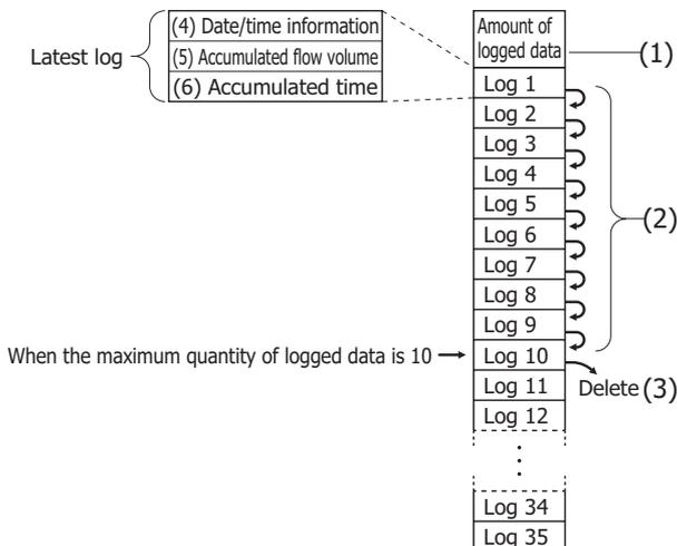
The maximum amount of logged data to use is specified on the **Settings** tab in the **FLWA (Analog Flow Totalizer)** dialog box.
