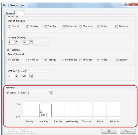
The preview shows the ON/OFF state for the output based on the settings configured on the parameter tabs as a time chart. The preview can be shown as a week or a day.
