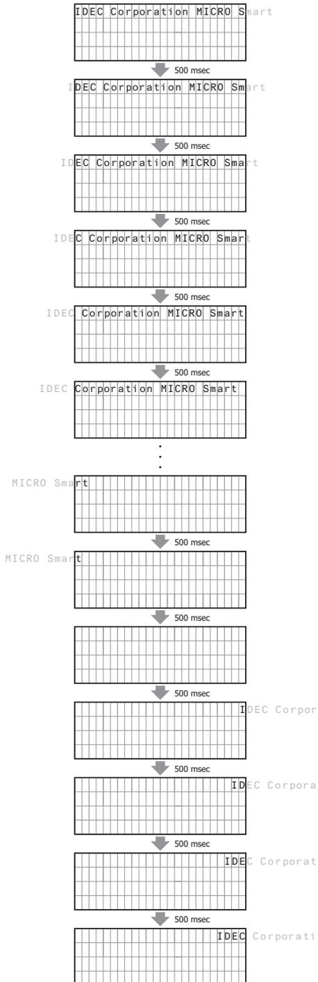
**When scrolling a text shorter than or equal to the specified area on the LCD**
