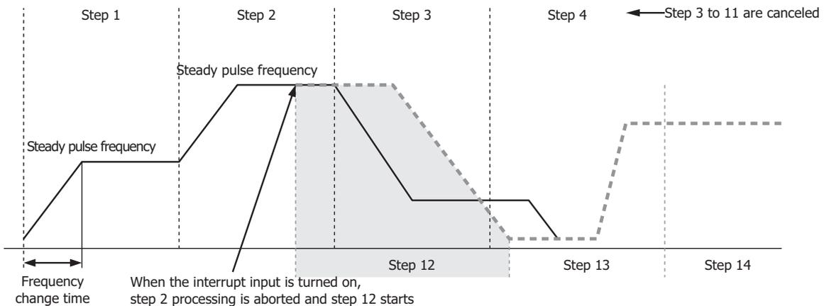
When the interrupt input turns on, step 2 which is currently outputting pulses is aborted, and pulse output starts from the step number set as the interrupt step number (step 12). When step 12 completes, pulses are output for the next step according to the set order of steps.
