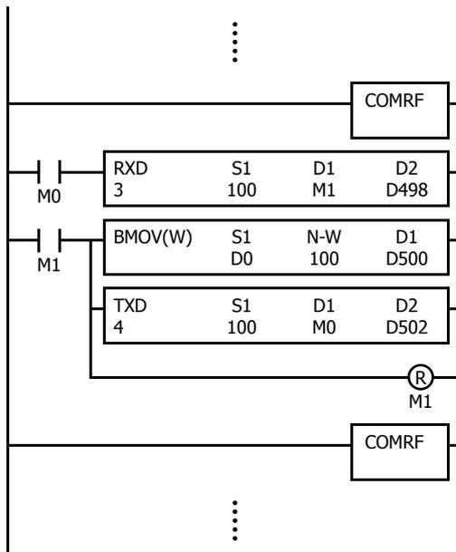
Before executing the RXD instruction, COMRF refreshes send and receive data of the expansion communication ports.
