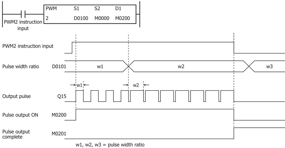
When the PWM2 instruction input changes from off to on, M0200 turns on and pulses with the width ratio configured by D0101 are output. If the value of D0101 changes during pulse output, pulses are output with the width ratio based on that value.
