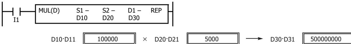
**Note:** In multiplication of double word data, the lower 32-bit data of the result is set to destination device D1·D1+1.
