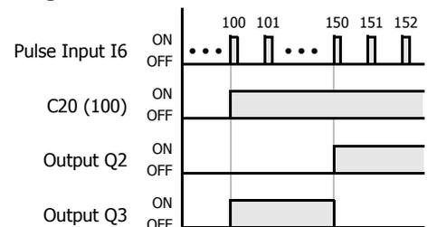
Output Q3 is on when counter C20 current value is between 100 and 149.
