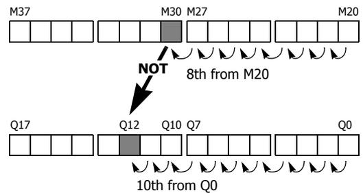
As a result, when input I0 is on, the ON/OFF status of internal relay M30 is inverted and moved to output Q12.
