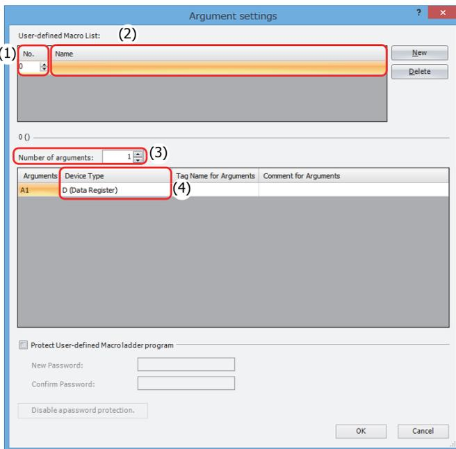
**Note:** You can prevent the settings in the **Argument settings** dialog box from being changed by selecting the **Protect User-defined Macro ladder program** check box and setting a password.
