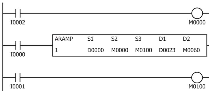
When I2 turns on, the initialization input (M0000) is turned on and the ARAMP instruction control register values are initialized
