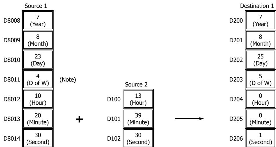
**Note:** D8011 in source 1 is not used for execution and does not need to be designated. The day of week is calculated automatically from the resultant year, month, and day, and stored to D203 of destination 1.
