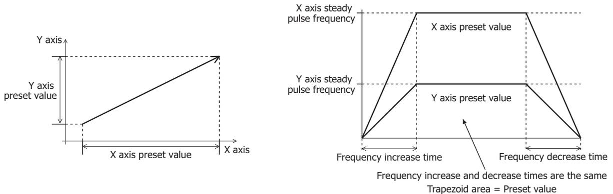
When the initialization input specified by S2 is turned on, the initial values configured in the WindLDR **RAMPL (Ramp Pulse Output with Liner Interpolation)** dialog box, on the **Common Settings** tab, are stored in the control registers.
