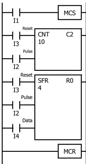
When input I1 is on, the MCS is not executed so that the counter and shift register are executed according to the actual status of subsequent inputs I2 through I4.
