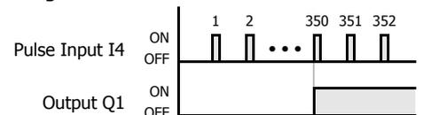
Output Q1 is turned on when counter C31 current value reaches 350 and remains on until counter C31 is reset.
