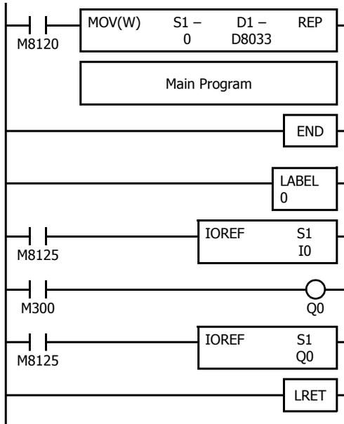
M8120 is the initialize pulse special internal relay.
