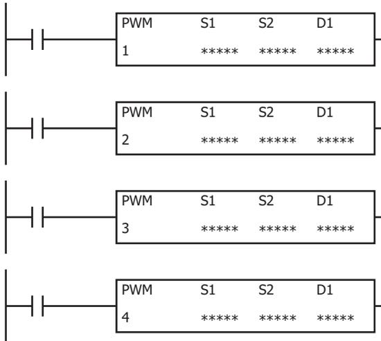
The PWM instruction outputs pulses of the specified frequency and duty cycle from the output.
