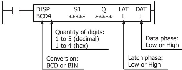
Displays the specified data on a 7-segment display.
