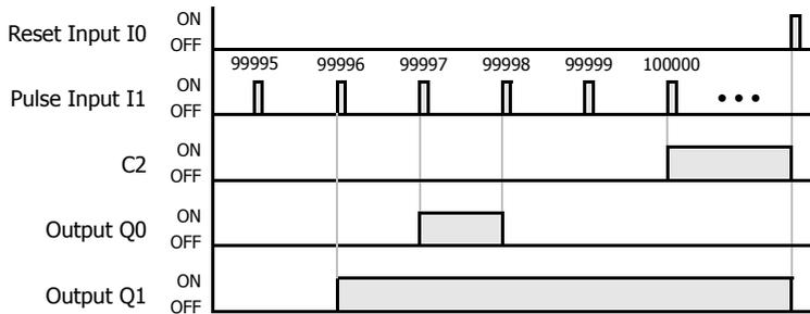
Output Q0 is on when counter C2 current value is 99,997.
