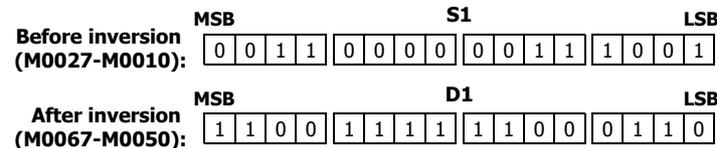
The ON/OFF statuses of the 16 internal relays M10 through M17 and M20 through M27 are inverted and moved to 16 internal relays M50 through M57 and M60 through M67. M50 is the LSB (least significant bit), and M67 is the MSB (most significant bit).
