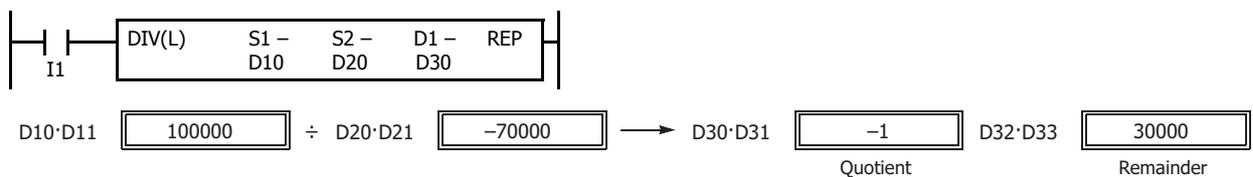
**Note:** Since the destination uses four word devices in the division operation of long data, data registers such as D7997 cannot be used as destination device D1. When using a bit device, such as internal relay for destination, 64 internal relays are required; so internal relay such as M7921 cannot be used as destination device D1.
