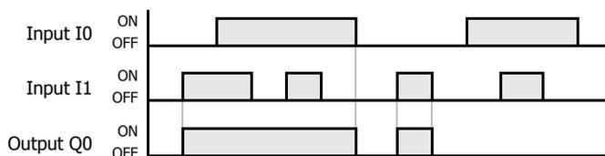
When input I0 is on, JMP is executed so that the subsequent output status is held.
