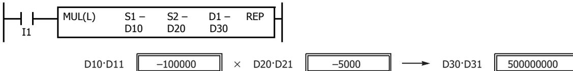
**Note:** In multiplication of long data, the lower 32-bit data of the result is set to destination device D1·D1+1.
