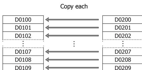
**Note:** Even if the data type is set to D (double word), L (long), or F (float), the data is copied from the first device in word units.
