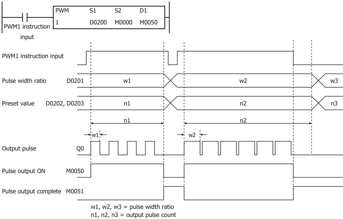
When the PWM1 instruction input changes from off to on, M0050 turns on and pulses with the width ratio configured by D0201 are output. When the number of pulses configured by D0202 and D0203 are output, pulse output stops. If the value of D0201 changes during pulse output, pulses are output with the width ratio based on that value.
