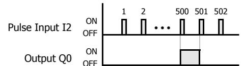
Output Q0 is on when counter C30 current value is 500.
