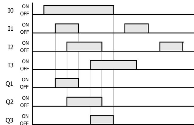
When both inputs I0 and I1 are on, output Q1 is turned on.
