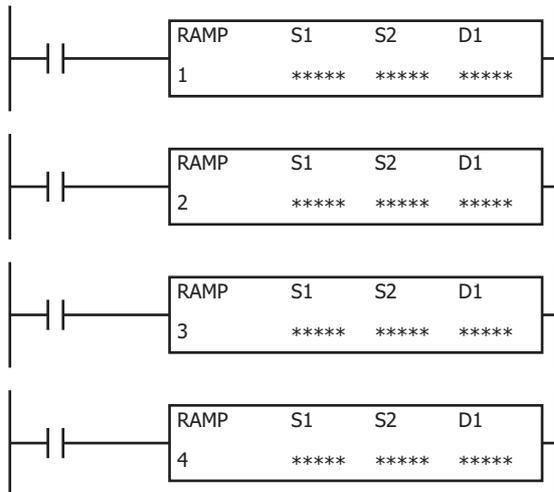
The RAMP instruction outputs pulses with a frequency change function.
