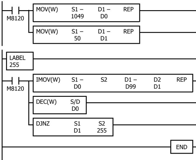
M8120 is the initialize pulse special internal relay.
