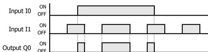
When input I0 is off, MCS is executed so that the subsequent input is forced off.
