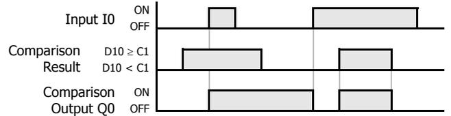
This program turns the output off when the input is off.
