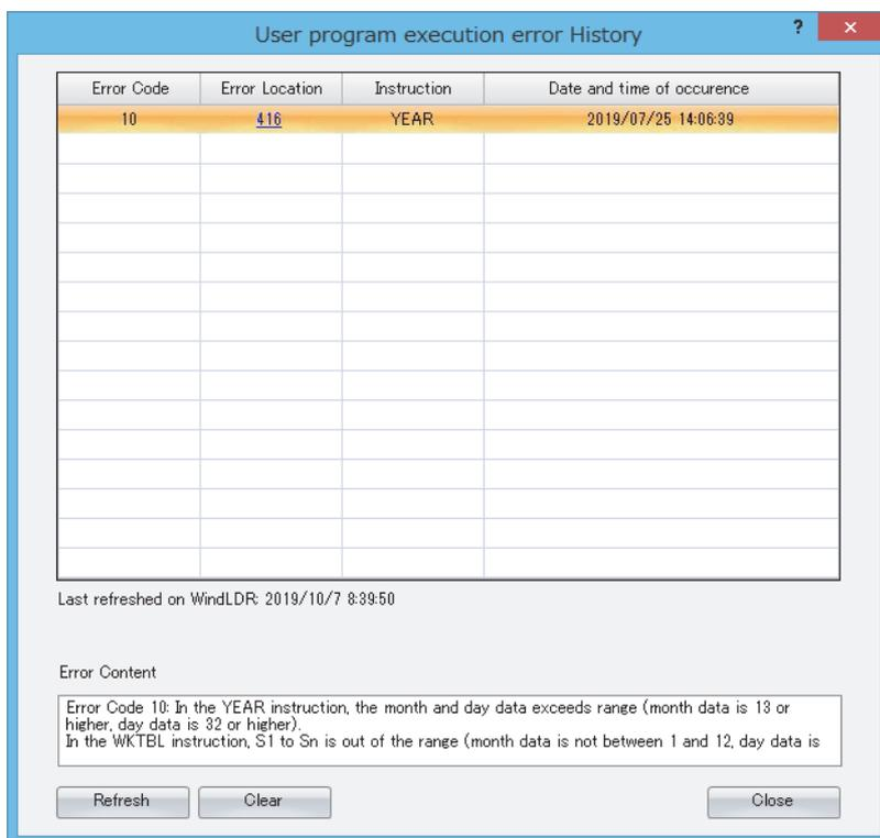
**Note:** If the ladder program on the FC6A Series MICROSmart is not the same as the ladder program displayed in the WindLDR Ladder Editor, search for the instruction symbol near the line number of the location where the error occurred.
