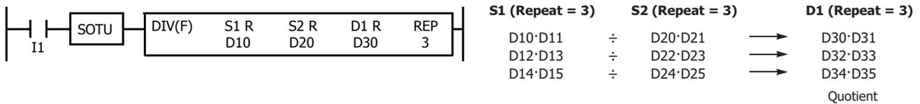
**Note:** When a user program execution error occurs in any repeat operation, special internal relay M8004 (user program execution error) and the ERR LED are turned on and maintained while operations for other instructions continues.
