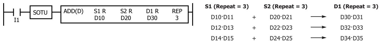
**Note:** Special internal relay M8003 (carry/borrow) is turned on when a carry or borrow occurs in the last repeat operation. When a user program execution error occurs in any repeat operation, special internal relay M8004 (user program execution error) and the ERR LED are turned on and maintained while operations for other instructions continues.
