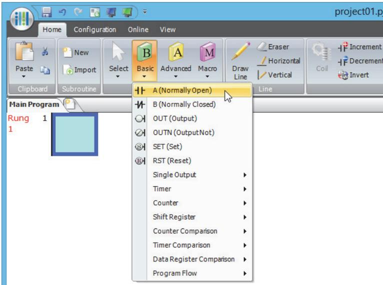
2. Move the mouse pointer to the first column of the first line where you want to insert a NO contact, and click the left mouse button.
