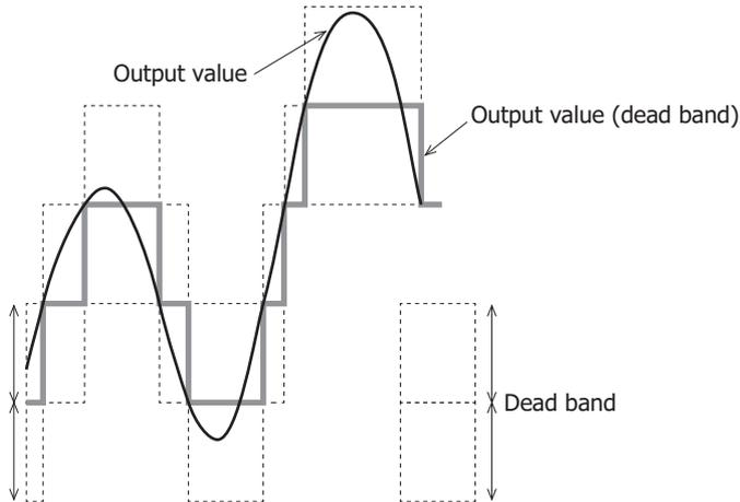
When the SCALE instruction is executed, it stores the value scaled in the first scan in output value (D1+0, D1+1) and updates the output value (dead band) (D1+2, D1+3).
