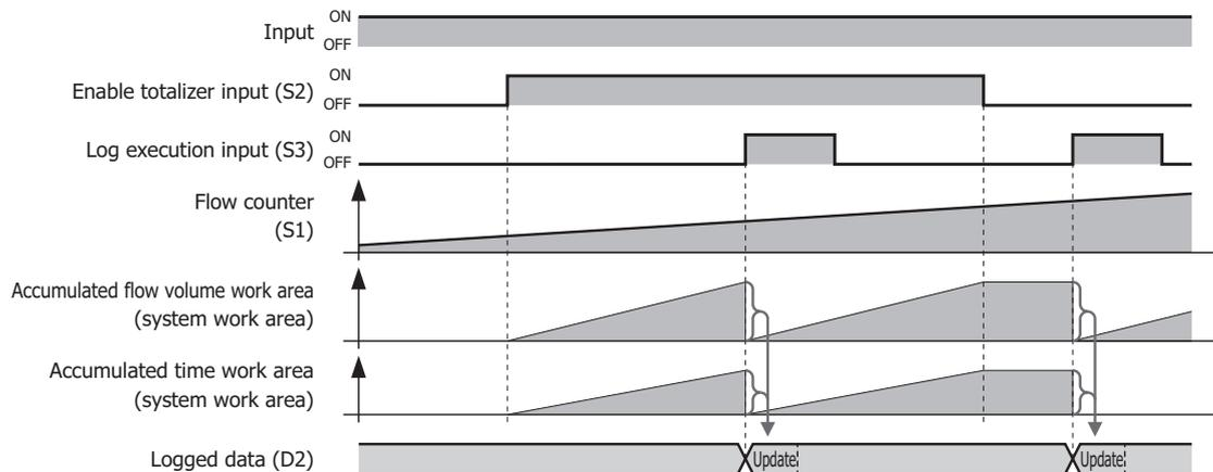
**Note:** For details on the log output function such as the operation immediately after the input is turned on, the operation when the enable totalizer input (S2) is once again turned on, and the logged data updating when the log execution input (S3) is turned on, see "Log Output Function" on page 27-23.
