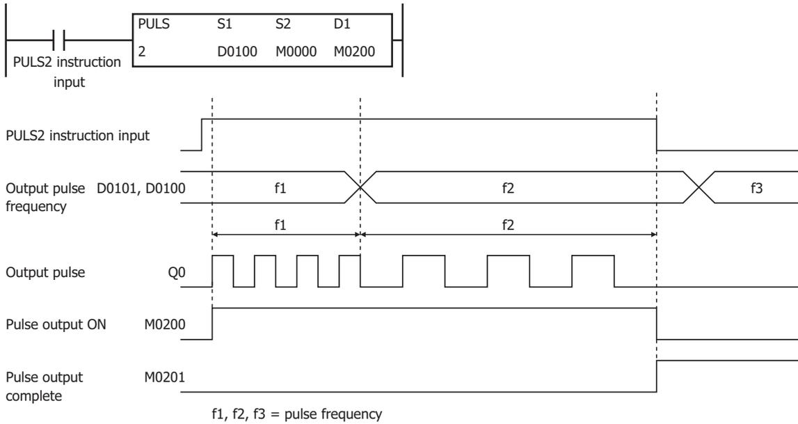
When the PULS2 instruction input changes from off to on, M0200 turns on and pulses with the frequency configured by D0101 and D0100 are output. If the value of D0101 and D0100 changes during pulse output, pulses are output with the frequency based on that value.
