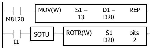
M8120 is the initialize pulse special internal relay.
