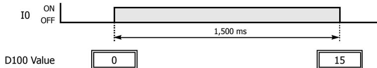
The following example demonstrates a program to measure the ON duration of input I0 and to use the ON duration as a preset value for 100-ms timer instruction TIM.
