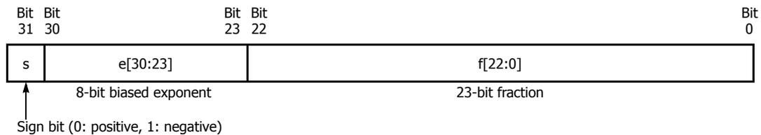
The table below shows the correspondence between the values of the three constituent fields s, e, and f and the value represented by the single precision format bit pattern.
