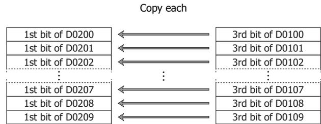
**Note:** Even if the data type is set to D (double word), L (long), or F (float), the bits are copied from the first device in bit units.
