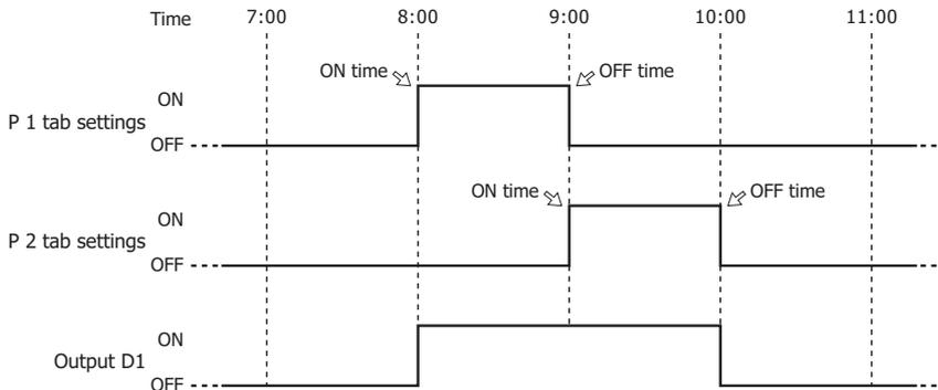
If **ON time** is 9:00 and **OFF time** is 10:00 on the **P 1** tab and **ON time** is 8:00 and **OFF time** is 9:00 on the **P 2** tab, the 9:00 setting is duplicated on the two tabs and **ON time** for the **P 1** tab is disabled. In this situation, the output is on from 8:00 to 9:00.
