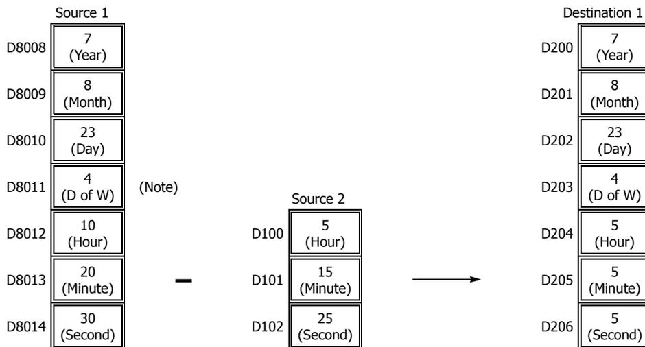
**Note:** D8011 in source 1 is not used for execution and does not need to be designated. The day of week is calculated automatically from the resultant year, month, and day, and stored to D203 of destination 1.
