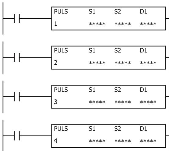
The PULS instruction outputs pulses of the specified frequency from the pulse outputs with a fixed duty cycle.
