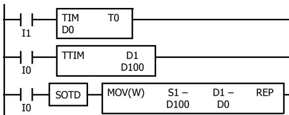
When input I1 is turned on, 100-ms timer T0 starts to operate with a preset value stored in data register D0.
