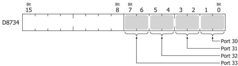
0 (00): The signal is on when the FC6A Series MICROSmart is set to run and off when stopped. While running, the signal is always on regardless of transmitting or receiving data. Set this value when it is necessary to indicate the run status.
