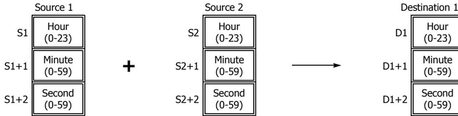
Hour data can be 0 through 23. Minute and second data can be 0 through 59.
