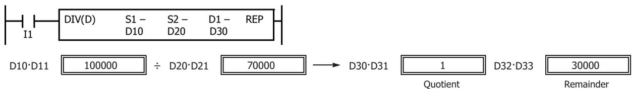
**Note:** Since the destination uses four word devices in the division operation of double-word data, data registers such as D7997 cannot be used as destination device D1. When using a bit device such as internal relay for destination, 64 internal relays are required; so internal relay such as M7921 cannot be used as destination device D1.
