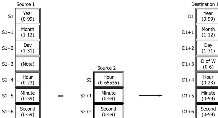
**Note:** Device S1+3 in source 1 is not used for execution and need not be designated.
