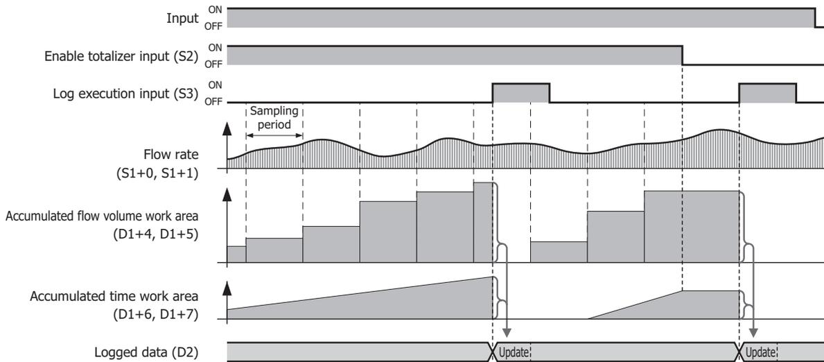
**Note:** For details on the log output function such as the operation immediately after the input is turned on, the operation when the enable totalizer input (S2) is once again turned on, and the logged data updating when the log execution input (S3) is turned on, see "Log Output Function" on page 27-13.
