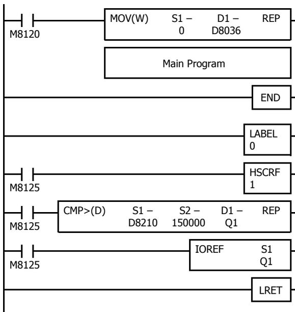
M8120 is the initialize pulse special internal relay.
