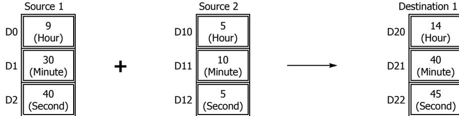
When the result exceeds 23:59:59, the resultant hour data is subtracted by 24, turning on special internal relay M8003 (carry).
