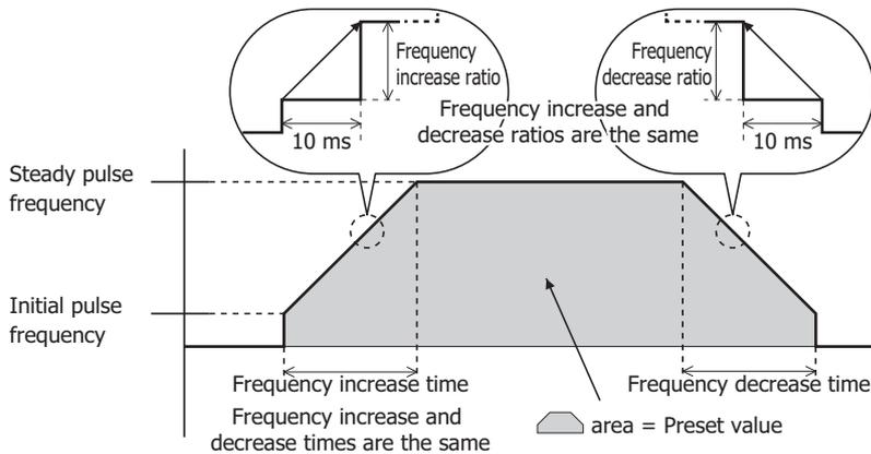
When the initialization input specified by S2 is turned on, the initial values configured in the WindLDR **RAMP (Trapezoidal Control)** dialog box, on the **Settings** tab, are stored in the control registers.
