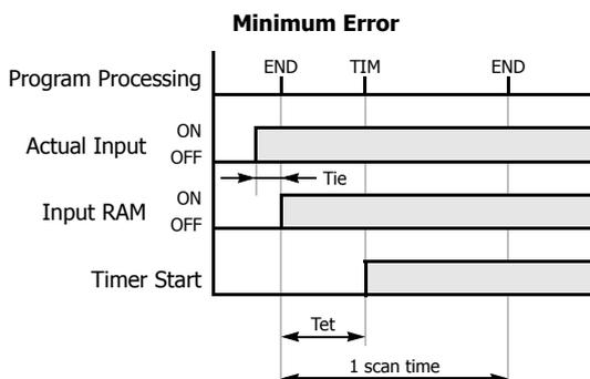
When the input turns on immediately before END processing, Tie is almost 0. Then the timer input error is only Tet (behind error) and is at its minimum.
