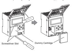
3. Take care with the vertical orientation of the analog cartridge and firmly push the cartridge connector onto cartridge slot 3 on the HMI module.
