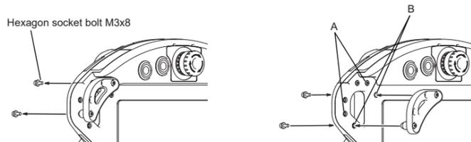
(1) Remove the two hexagon socket head bolts on the back of the main unit.
