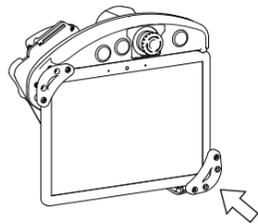
(4) Slide the slide arm so that the four spacers touch the tablet. to hold the tablet securely. Insufficient holding may cause the tablet to fall.
