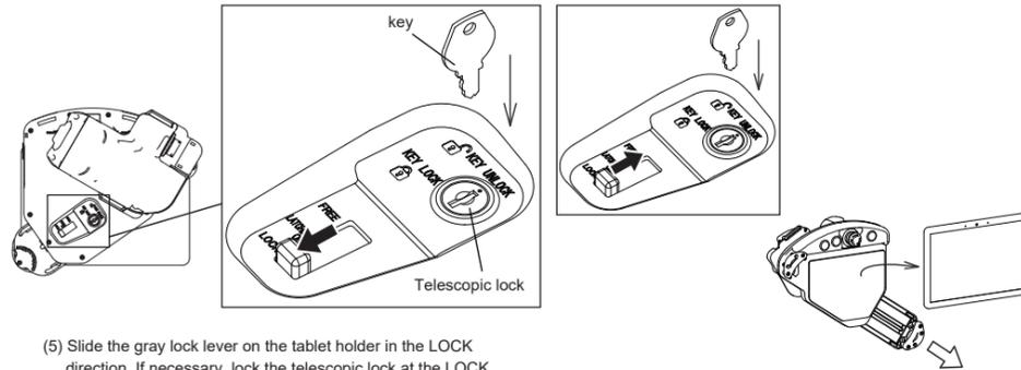
(5) Slide the gray lock lever on the tablet holder in the LOCK direction. If necessary, lock the telescopic lock at the LOCK position and remove the key. The lock lever is fixed at the LOCK position. Do not operate the telescopic lock in the FREE position. It will be the cause of the failure.
