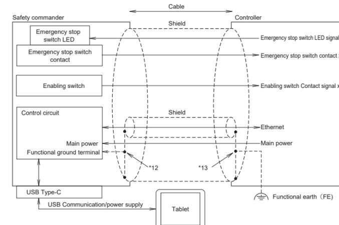
\*12 Connect both shields to the functional earth terminal.
