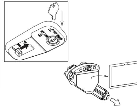
(1) If the key is locked, open it with the key, and then slide the gray lock lever to the FREE position. The weight of the tablet may cause the slide arm to open and the tablet to fall at that time.
