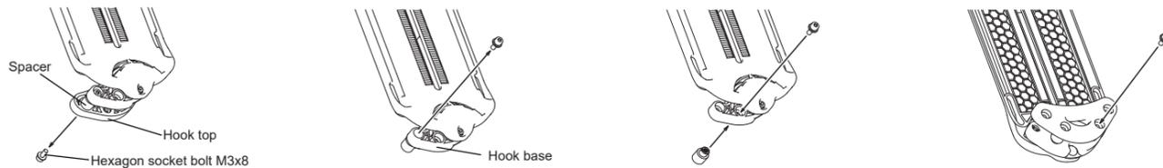
(1) Remove the hexagon socket bolt (hex wrench size: 2.5) on the front side of the hook.
