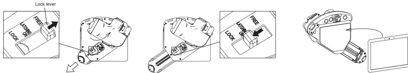
(1) Rotate the grip unit. Slide the gray lock lever on the tablet holder in the FREE direction and loosen the slide arm.
