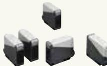
Universal voltage types operate on 24-240V AC and 12-240V DC. DC power types operate on 12-24V DC. Four sensing methods (through-beam, polarized retro-reflective, diffuse-reflective, and background suppression).
