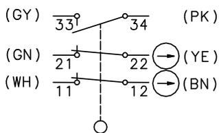
The colour allocation refers to the plug-in-cables which we have in our range.
