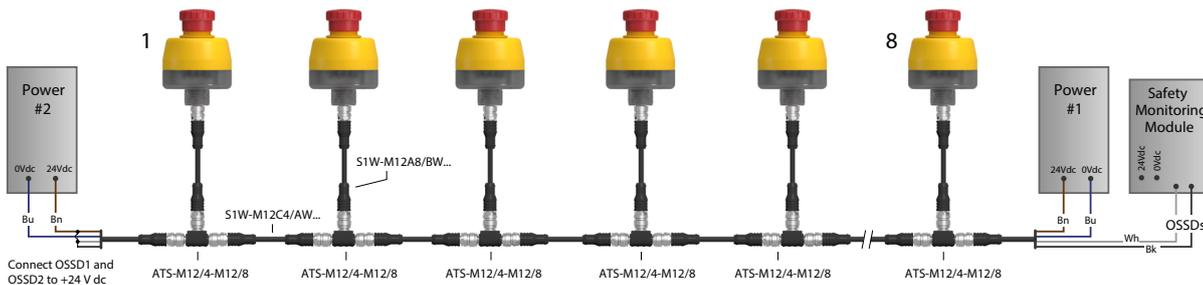
Figure 13. Option 2: Replace the terminator with a power supply. The OSSD1 and OSSD2 wires at power supply #2 must be connected to +24 V DC. If available, set the power supplies for parallel output.
