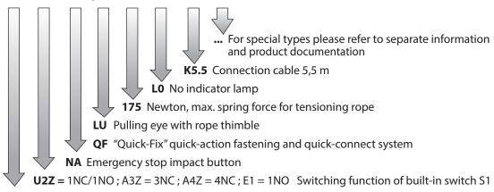
**SR** Safety rope pull switch (switching device range)
