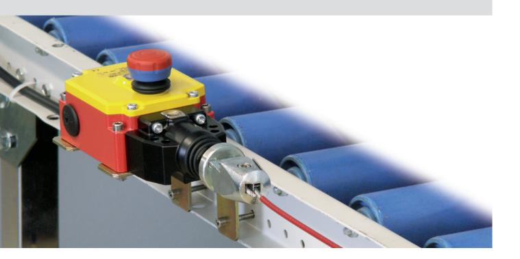
The SR and SRM series of safety rope pull switching devices developed and manufactured by BERNSTEIN AG are designed and approved in accordance with the standards IEC 947-5-5, IEC 60947-5-5 and ISO 13850. On actuation or in the event of cable breakage, the emergency stop switching device locks automatically and can only be reset to its initial setting by using the resetting device on the switch.
