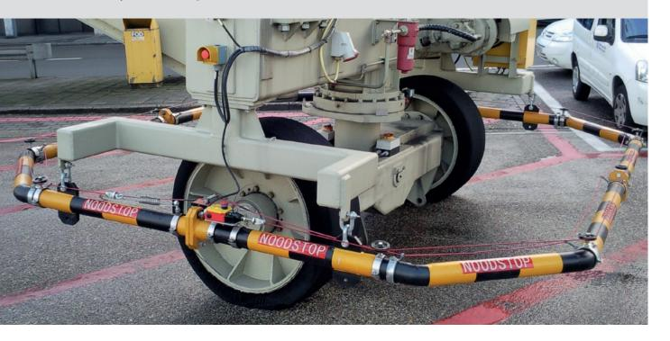
The BERNSTEIN safety rope pull switch is used in boarding bridges designed to ensure passengers can safely board and alight aircraft at airports throughout the world.
