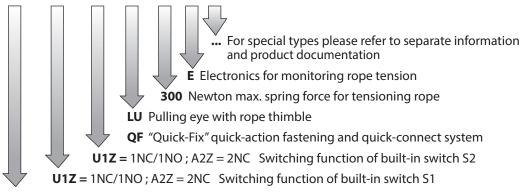
**SRM** Safety rope pull switch (switching device range)
