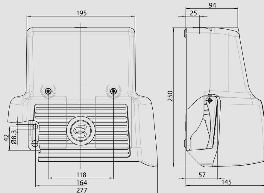
Product selection Single-pedal foot switch with enabling function F1
