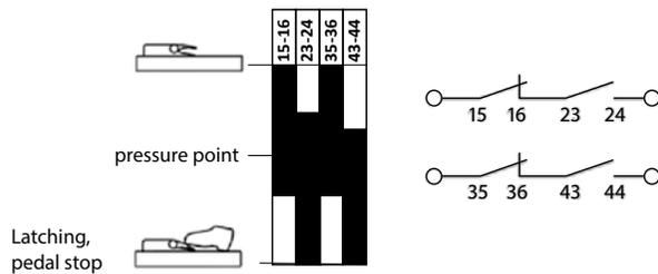
Due to the series connection of the overlapping contacts, an OFF-ON-OFF function is achieved as with the enabling function. However, when the pedal is returned from the 3rd level, the 2nd level is always passed through as well. For this reason, the foot switches with safety latch and manual release are only available with a reset button. When this button is pressed, the 2nd level is passed through within a few milliseconds.
