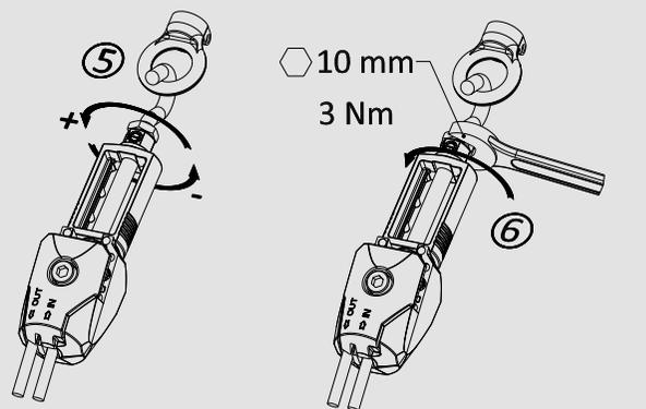
Secure the Quick-Fix quick-release head with an Allen screw SW 4, complete the assembly.
