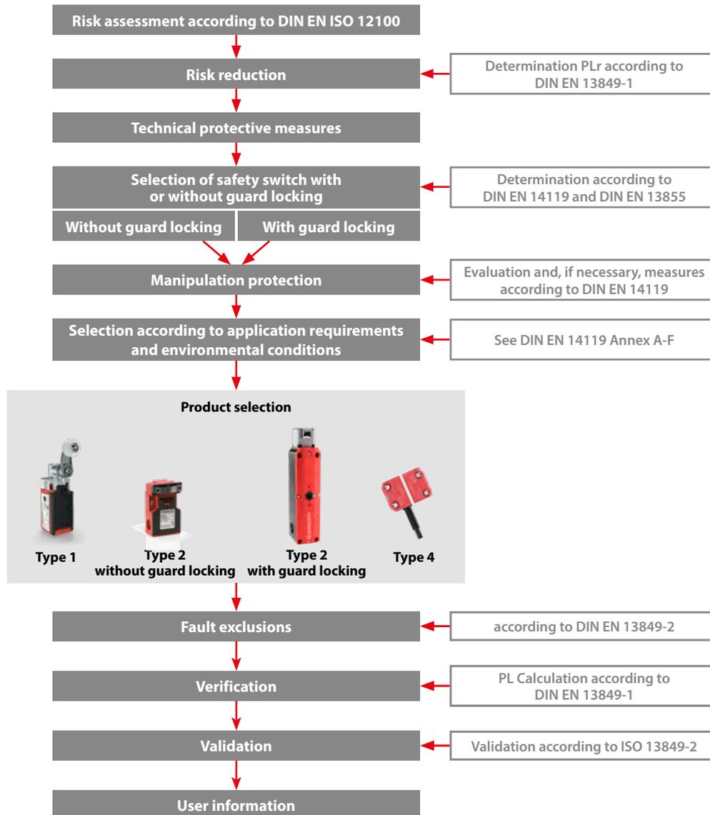
The overview on the right and the following explanations on pages 8–13 describe a procedure for selecting the correct products for position monitoring and, if necessary, guard locking of safety gates and hoods and for implementing their integration in the safety-related part of the control system.
