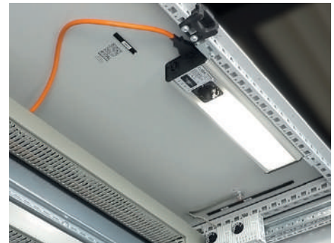
Assembly on 35 mm top hat DIN rails
