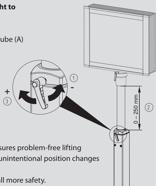
The integrated gas pressure spring ensures problem-free lifting of the visualisation unit and prevents unintentional position changes after releasing the clamping lever.
