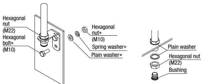
The parts marked with \* are not supplied and should be prepared by the user.
