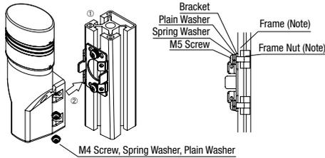
Note: See table below for typical examples of frames and nuts. Consult the manufacturer of the frame for the installation method of the frame nut.
