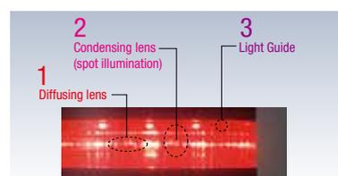
By combining a diffusing lens, which diffuses the light broadly, with a condensing lens, a super bright area is created enabling high visibility. Also, the illumination through the light guide enhances the visibility when the SignalLight is viewed from below.
