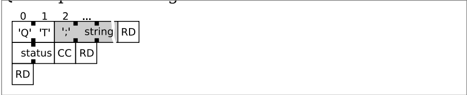
Figure 8.7.4.1: QT command Request and Response
