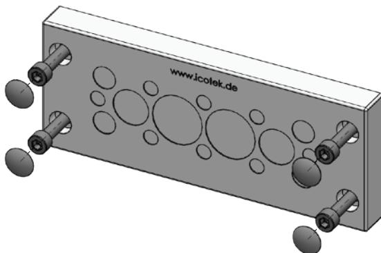
When fastening from the front by means of screws, the openings at the screw heads can be closed with the **cover plugs B** in black (order no. 99200) or **cover plugs C** in grey (order no. 99201). The cover plugs can only be used for M5 DIN 912 screws.
