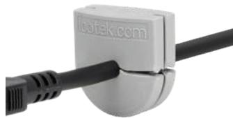
With the UT split cable grommet, cables with and without connectors can be easily and cost-effectively inserted into an enclosure and sealed with IP54. All that is required for installation is a U-shaped cut-out into which the fitted grommet is inserted. The UT can be used universally for cables (compressed air hoses, glass fibre tubes, etc.) with a diameter of 4 to 11 mm. The wall thickness of the housing can be from 1 to 4 mm.
