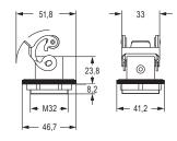
Angled bulkhead mounting housings,1 stainless steel lever
