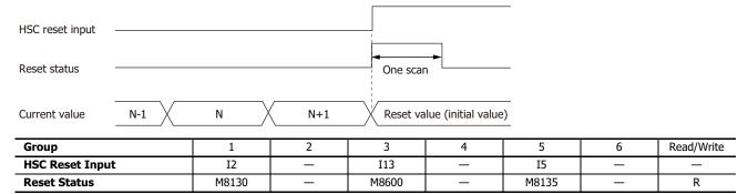
To use the reset input with the group 1, group 3, or group 5 single-phase high-speed counter, use I2, I13, or I5. When not using I2, I13, or I5 as an external reset input, they can be used as normal input.
