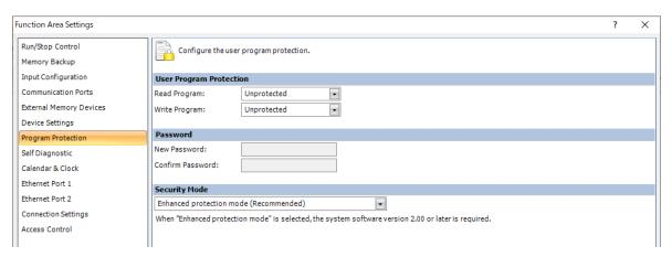
2. Under User Program Protection, select required protect modes for Read Program and Write Program in the pull-down list.
