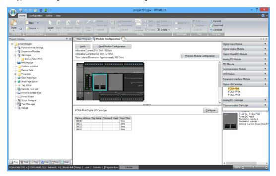
**2.** Click the inserted digital I/O cartridge in the module configuration area and click **Configure**. The configuration dialog box that corresponds to the digital I/O cartridge is displayed.
