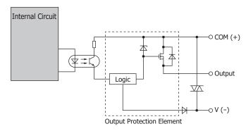
(The overcurrent detection circuit has been omitted.)
