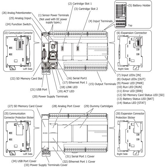
The content in brackets is the LED indicator name on the FC6A Series MICROSmart.
