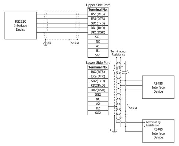
The serial communication module is equipped with two serial ports, and serial communication can be performed using both serial ports simultaneously. RS-232C or RS-485 can be selected and used for each port.
