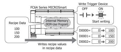
To write the recipe values in recipe data saved in FC6A Series MICROSmart internal memory (ROM-Range) to devices
