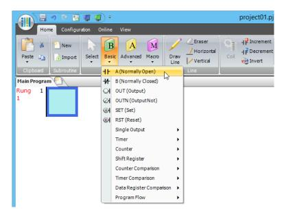
**2.** Move the mouse pointer to the first column of the first line where you want to insert a NO contact, and click the left mouse button.
