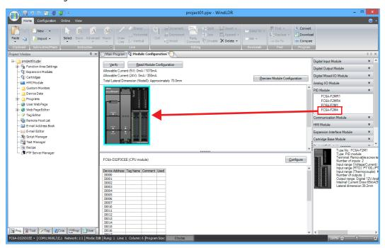
The expansion module or cartridge is inserted into the module configuration area.
