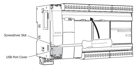
2. Open the USB port cover in the direction of the arrow.
