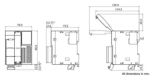
\*1 The above drawing is for the screw fastened type. Dimensions for the push-in type are given in [ ].
