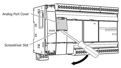
2. Lift up the analog port cover in the direction of the arrow to remove it.
