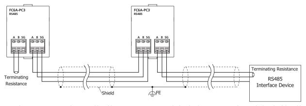
**Note:** When communication quality is unstable, add terminating resistance matched to the characteristic impedance to both ends of the cable. Use resistance with a rating of 1/2 W or higher.
