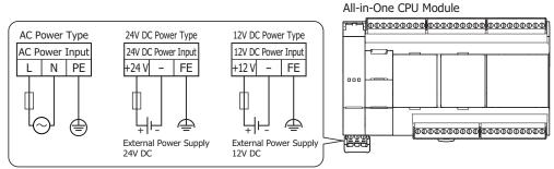
The power supply specification of the Plus CPU module is the 24V DC power type only.
