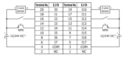
\*1 24V DC for products with a version number lower than V400. For details on the version number of modules, see "Checking the Version Number" on page 2-1.
