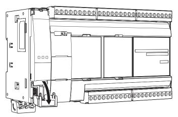
**Note:** To remove the USB cover, first open the cover in step 2, and then apply force in that same direction to remove the cover.
