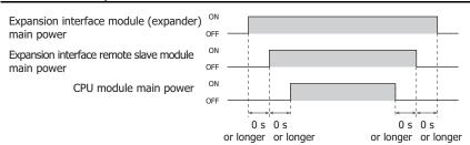
If the order to turn on the power supply is wrong, the expansion interface modules (remote master/slave) along with the connected expansion modules can be initialized by turning on M8320 (Initialize Expansion Interface Remote Master/Slave Modules).
