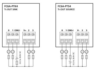
L) Rated Load: 12 to 24V DC/0.1 A
