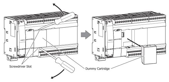
**2.** Take care with the vertical orientation of the analog I/O cartridge and firmly push the analog I/O cartridge connector onto cartridge slot 1 on the CPU module.
