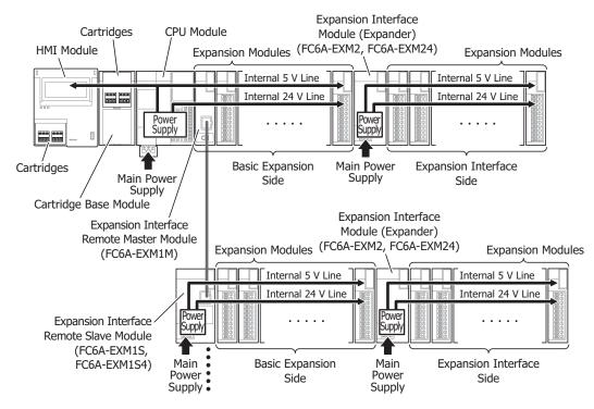
The internal power supply current that can be supplied to the expansion modules on the basic expansion side, HMI module, cartridge base module, and cartridges depends on the module supplying the power. Ensure that the total amount of current for the expansion modules on the basic expansion side, HMI module, cartridge base module, and cartridges does not exceed the limit of the internal power supply that can be supplied.
