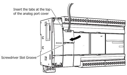
Note: Take care with the orientation of the analog port cover. The groove to insert the screwdriver goes on the bottom.
