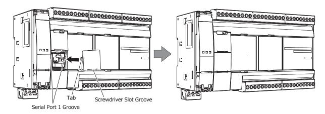
**Note:** Take care with the orientation of the serial port 1 cover. The groove to insert the screwdriver goes on the bottom.
