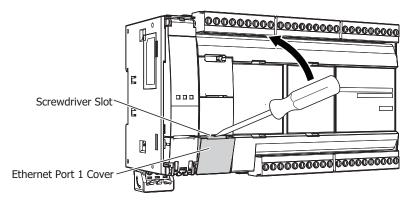
2. Lift the Ethernet port 1 cover straight up in the direction of the arrow to remove it.
