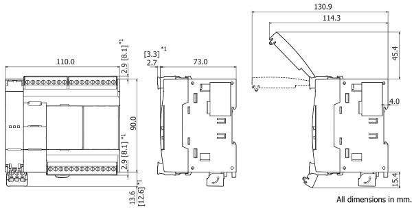
$<sup>^{*1}</sup>$  The above drawing is for the screw fastened type. Dimensions for the push-in type are given in [ ].
