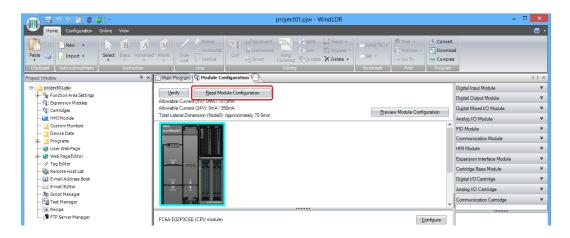
The configuration of expansion modules and cartridges connected to the CPU module is displayed in the module configuration area.
