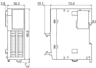
\*1 9.3 mm when the hook is pulled out.
