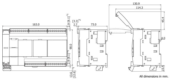
$^{*1}$  The above drawing is for the screw fastened type. Dimensions for the push-in type are given in [ ].
