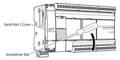
**2.** Lift the serial port 1 cover straight up in the direction of the arrow to remove it.
