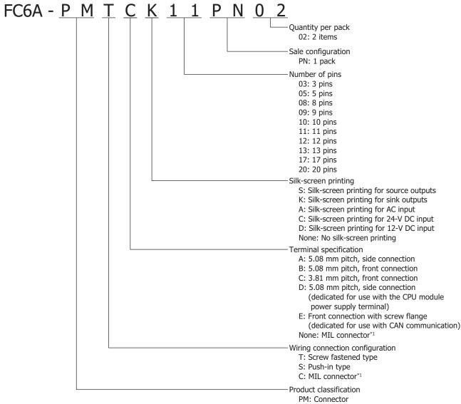
\*1 The type number for the MIL connector starts with "FC4A-" instead of "FC6A-".
