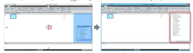
• If a floating window is dropped on the [1] (Docking) icon, it is docked to WindLDR's left, right, top, or bottom frame or a docked window.
