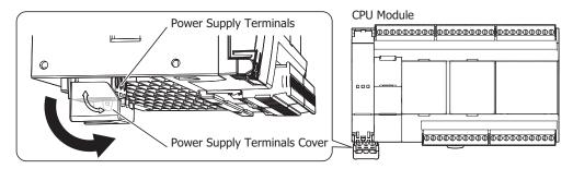
Rotate the power supply terminals cover until it touches the CPU module to unlock it, and then remove the power supply terminals.
