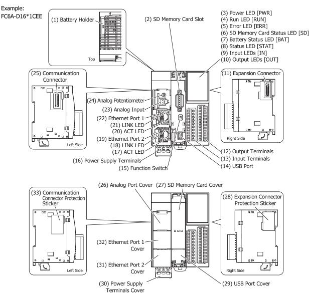
The content in brackets is the LED indicator name on the FC6A Series MICROSmart.
