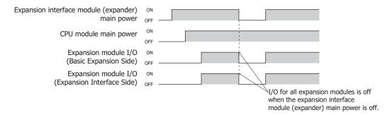
• If the expansion interface module (expander) main power supply is on and the CPU module main power supply is off, the expansion modules on the expansion interface side are set to the reset status. Please note that during the reset status, the analog I/O module and PID module LED indicators are on. This is not a malfunction.
