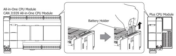
2. Remove the dead backup battery from the battery holder.
