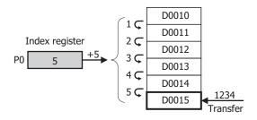
Values stored in the index registers is 32-bit and its data type is L (long). Index registers can directly specified as source and destination devices in MOV(L), ADD(L), SUB(L), and MUL(L) instructions and values in index registers can be moved or manipulated.
