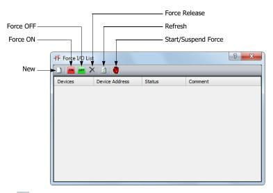
3. Click the New button and type an input or output number under Device in the list.
