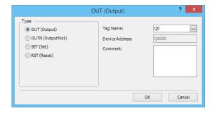
A NO output coil of output Q0 is programmed in the right-most column of the first ladder line. This completes programming for rung 1.
