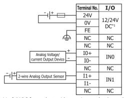
\*1 24V DC for products with a version number lower than V400. For details on the version number of modules, see "Checking the Version Number" on page 2-1.
