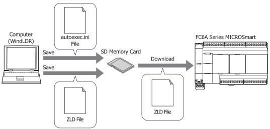
While the ZLD file saved to the SD memory card is being downloaded, CPU module operation stops. When the ZLD file is set to download the CPU module system software, the software is reset in order to rewrite the system software.
