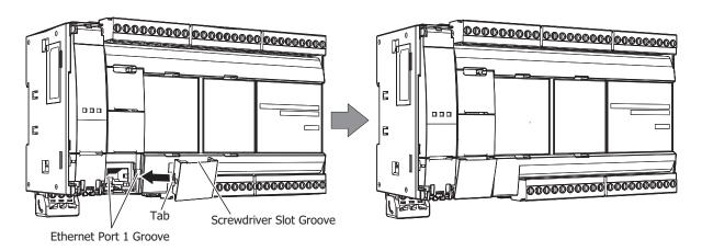
Note: Take care with the orientation of the Ethernet port 1 cover. The groove to insert the screwdriver goes on the bottom.
