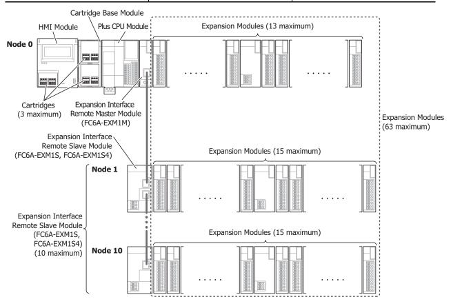
Maximum number of expansion modules: 63 Maximum number of expansion cartridges: 3
