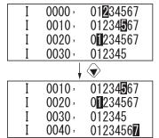
Shows the on/off state of the inputs (I). Inverted inputs are on state.
