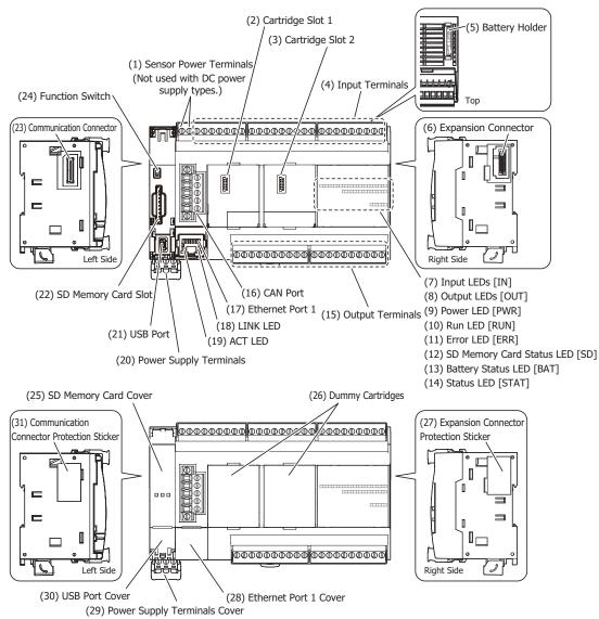
The content in brackets is the LED indicator name on the FC6A Series MICROSmart.
