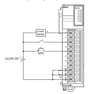
\*1 24V DC for products with a version number lower than V400. For details on the version number of modules, see "Checking the Version Number" on page 2-1.
