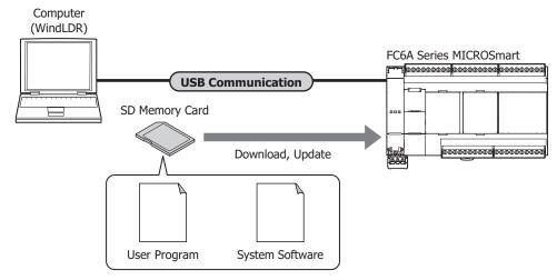
■ Read and write files on the SD memory card using WindLDR's Data File Manager
