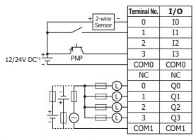
\*1 24V DC for products with a version number lower than V400. For details on the version number of modules, see "Checking the Version Number" on page 2-1.
