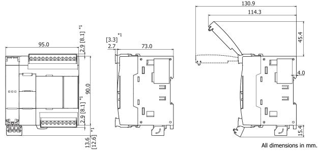
$<sup>^{*1}</sup>$  The above drawing is for the screw fastened type. Dimensions for the push-in type are given in [ ].
