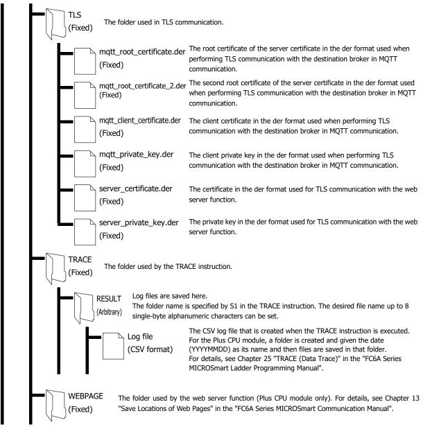
Note: The following group of four files is referred to as the files for MQTT Basic Settings.
