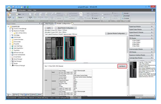
3. In the configuration dialog box, configure the parameters for the expansion module or cartridge.
