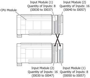
• When the positions of an analog I/O module or analog I/O cartridge are changed, the configured parameters are also moved. However, the device addresses in the program are not replaced.
