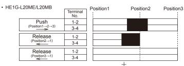
Emergency stop pushbutton switch : 2NC contacts (Terminal No.5-6 and 7-8) (HE1G-L20ME) Momentary pushbutton switch : 2NO contacts (Terminal No.5-6 and 7-8) (HE1G-L20MB)
