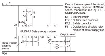
Note: Use the monitoring device(Safety relay module) provided the capavility to detect a cross short circuit. The insulation of the cable has to withstand environmental influences. If a control device other than the one shown in the draft is used, the used control device has to be equipped with a cross short circuit monitor.
