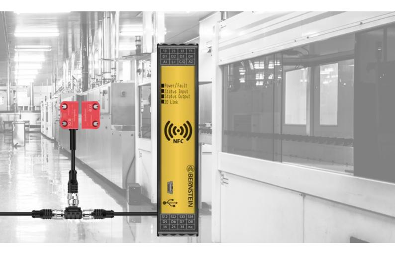
With the integrated diagnostic channel, all (non-safety) relevant status information of the connected sensors (SRF-5) and emergency stop devices (SEU) is transmitted to the machine control via a diagnostic device or the safe controller SCR DI – even in a series connection. In addition, the SCR DI provides its own diagnostic data. Three redundant, safe relays allow direct switching of loads with up to 6 A per enabling path.
