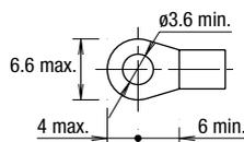
Dimensions for installing insulated tube
