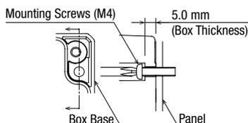
2. Installing the FB series from the rear
