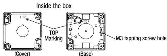
Installation using tapping screw hole inside the enclosure
