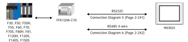
• MICREX-SX Series (Connects to Loader Connection Connector on the CPU unit)
