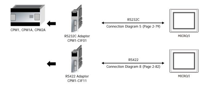
• SYSMAC C series (Connects to the Link Interface on the CPU unit)
