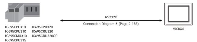
● Rx3i Series (Connects to Communication Coprocessor Module (IC695NIU001))
