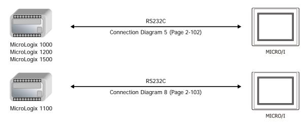
• MicroLogix 1500 (Connects to D-sub 9-pin Connector on the CPU unit)
