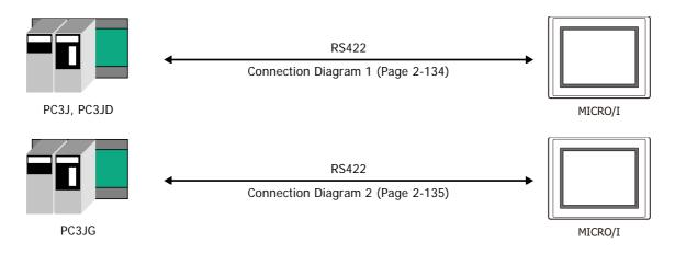
It connects with the Built-in Link port of a CPU unit.
