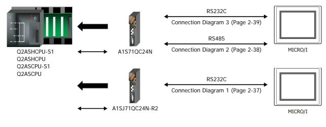
• MELSEC-Q Series (Connects to the CPU unit Programming Port)
