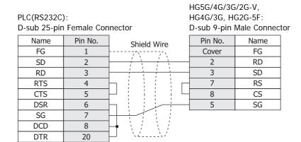
PLC(RS232C): HG5G/4G/3G/2G-V, D-sub 25-pin Female Connector HG4G/3G, HG2G-5F/-5T, HG1G: Terminal block Name Pin No. Shield Wire FG Pin No. Name 1 SD 2 2 RD SD RD 3 1 4 3 RS RTS 5 4 CS **CTS** 5 SG DSR 6 SG 7 DCD 8 DTR 20
