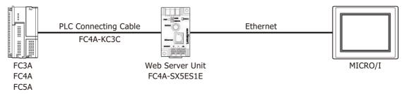
● FC5A MICROSmart (Connects to Ethernet port of the FC5A-D12\*1E)
